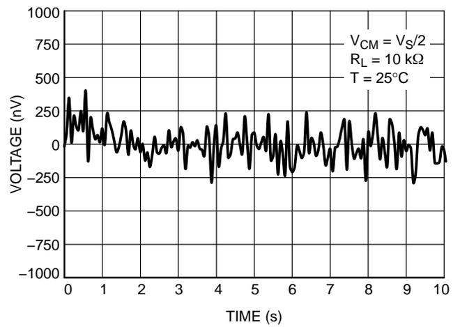
Figure 14. 0.1 Hz to 10 Hz Noise
