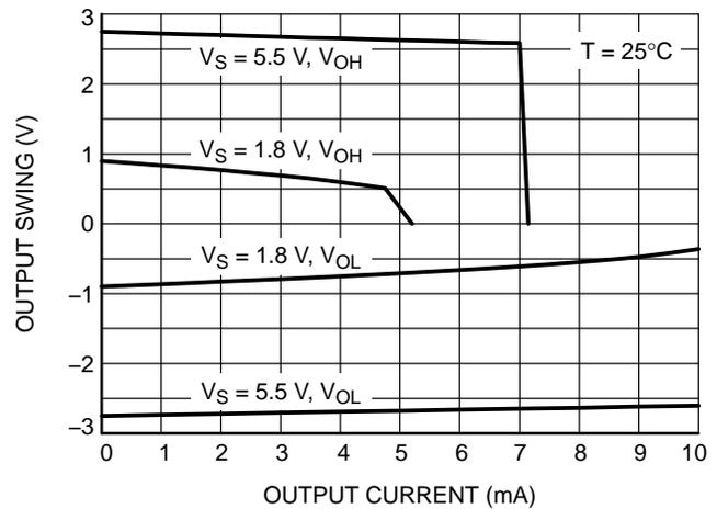
**Figure 4. Output Voltage Swing vs. Output Current**
