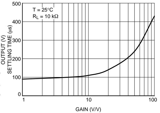
Figure 12. Settling Time to 0.1% vs. Closed-Loop Gain
