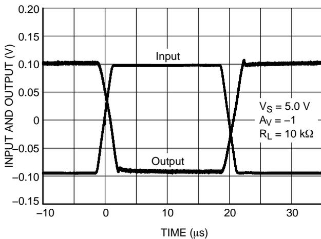
Figure 9. Small Signal Step Response
