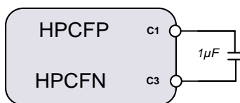
Figure 41: Charge Pump Flying Capacitor
