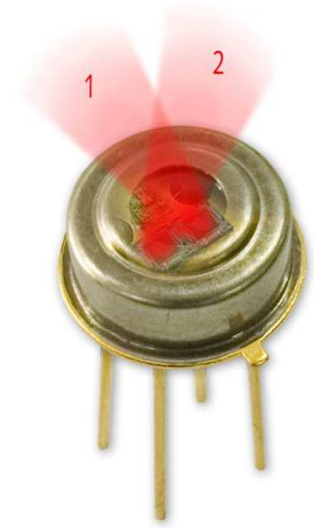
Figure 30: Identification of zone 1&2 relative to alignment tab
