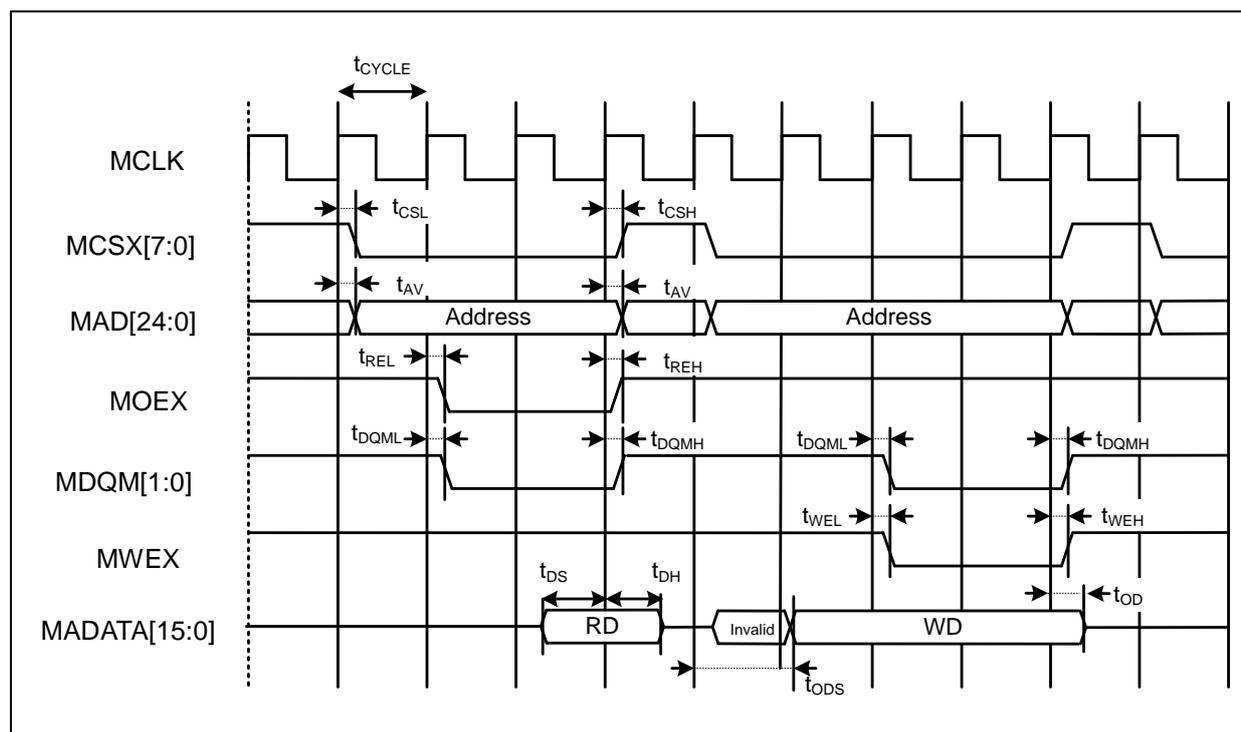
• Multiplexed Bus Access Asynchronous SRAM Mode
