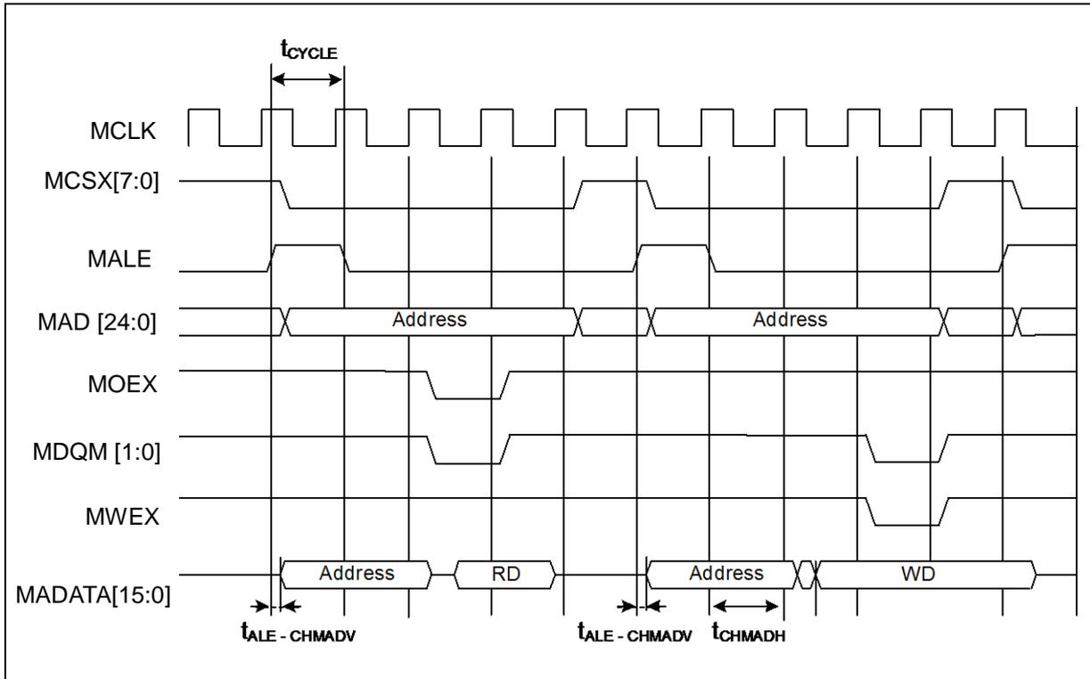
• Multiplexed Bus Access Synchronous SRAM Mode
