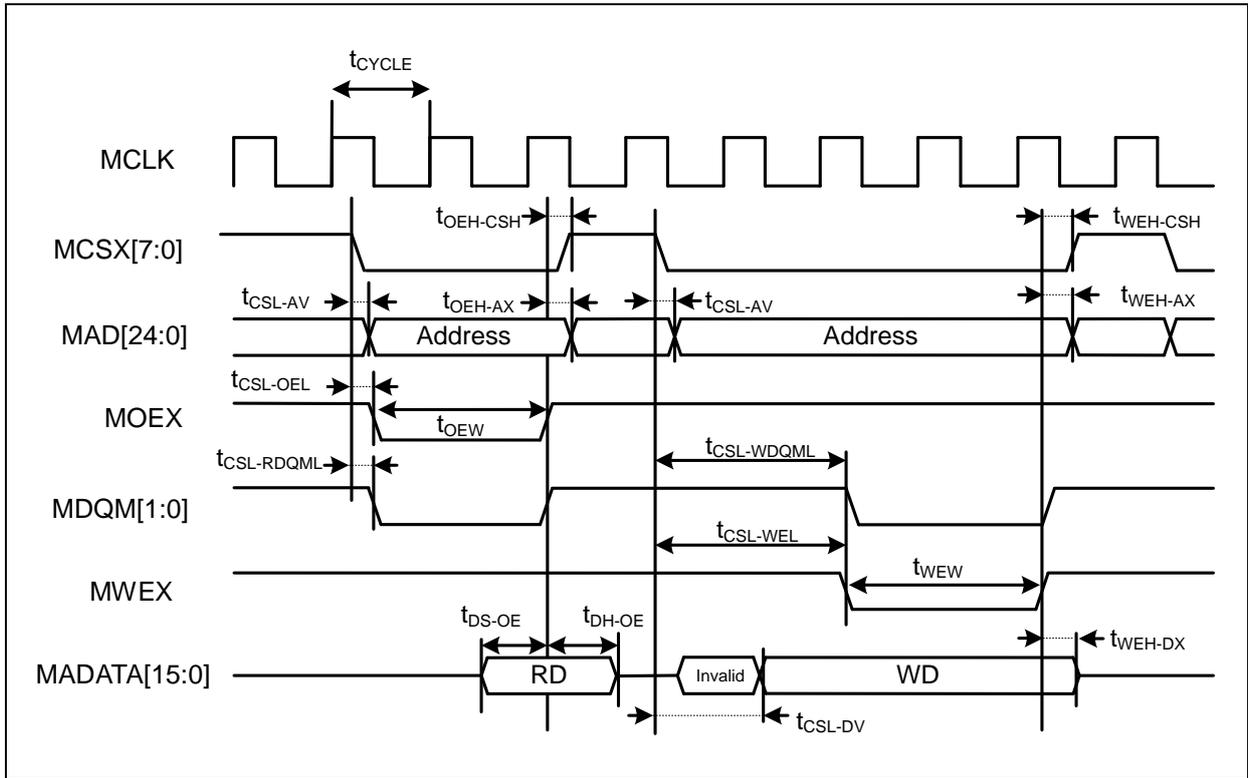
• Separate Bus Access Synchronous SRAM Mode
