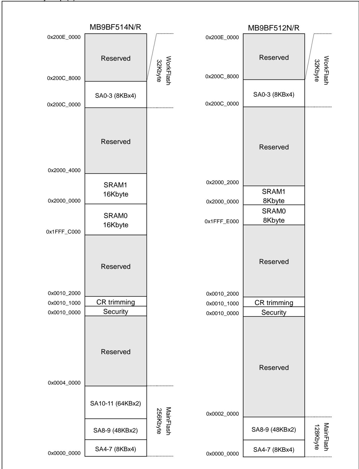
\*: See "MB9B510R/410R/310R/110R Series Flash programming Manual" for sector structure of Flash.
