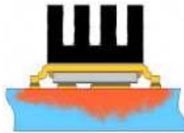
⑦ Mounted to a PCB with a thin gap filler and heat sink. (still air)
