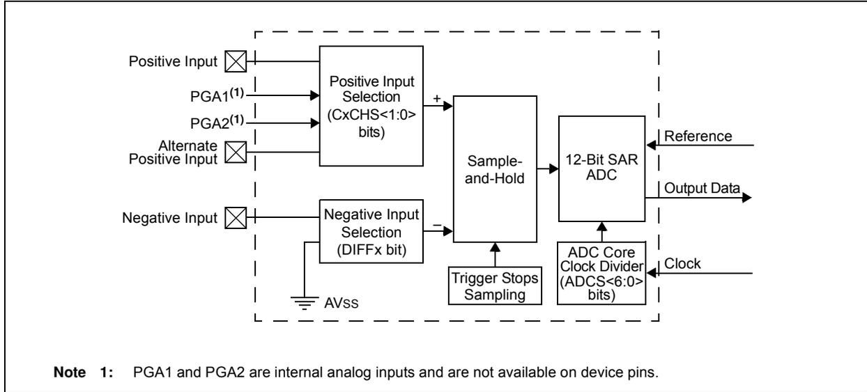
**FIGURE 19-3: SHARED ADC CORE BLOCK DIAGRAM**
