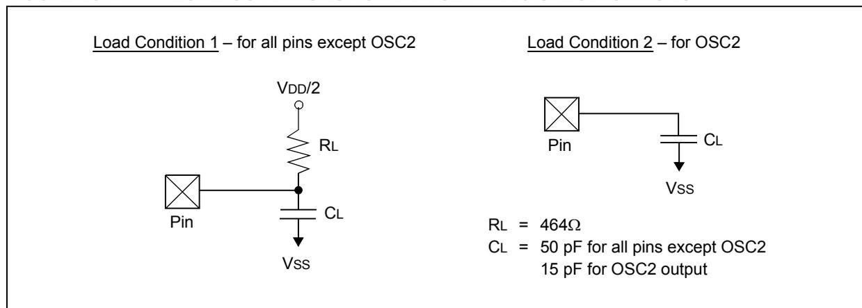
**TABLE 25-16: CAPACITIVE LOADING REQUIREMENTS ON OUTPUT PINS**
