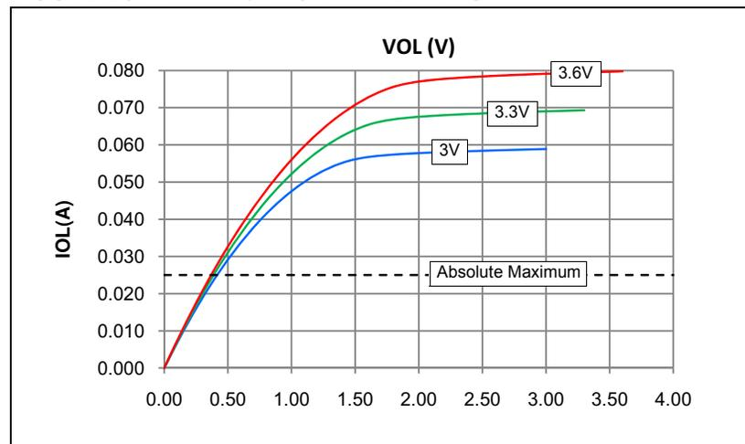
**FIGURE 26-5: TYPICAL I<sub>PD</sub> CURRENT @ V<sub>DD</sub> = 3.3V**
