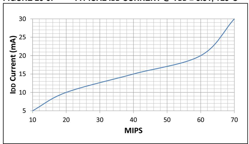
**FIGURE 26-8: TYPICAL I<sub>IDLE</sub> CURRENT @ V<sub>DD</sub> = 3.3V, +25°C**
