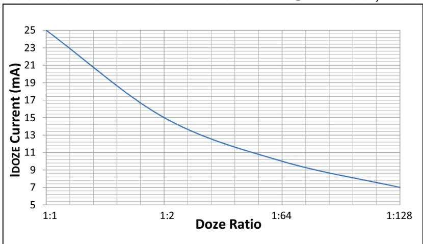
**FIGURE 26-6: TYPICAL I<sub>DD</sub> CURRENT @ V<sub>DD</sub> = 3.3V, +25°C**
