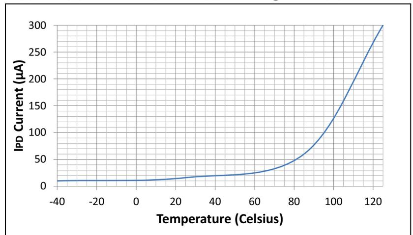
**FIGURE 26-7: TYPICAL I<sub>DOZE</sub> CURRENT @ V<sub>DD</sub> = 3.3V, +25°C**
