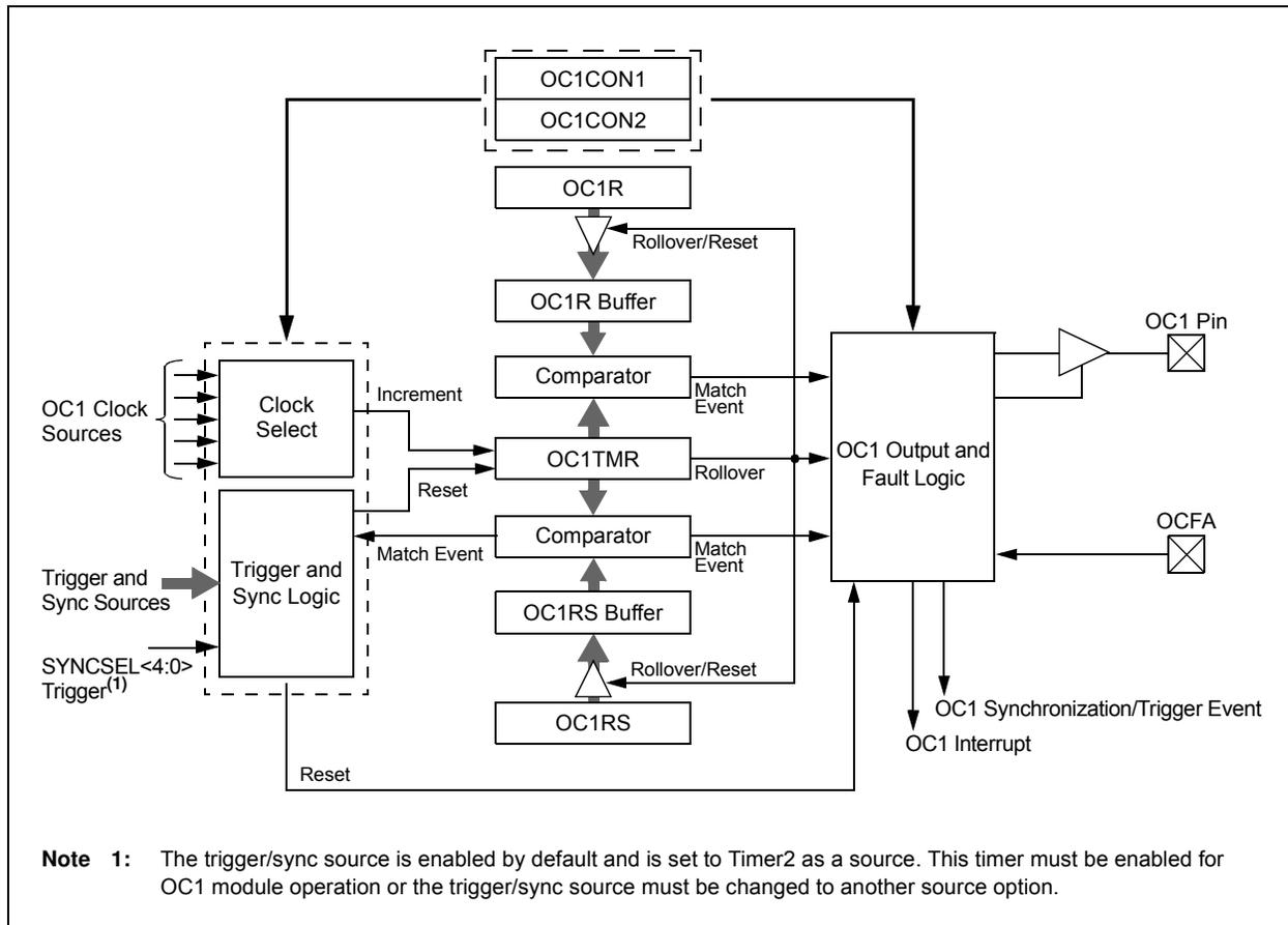
**Note 1:** The trigger/sync source is enabled by default and is set to Timer2 as a source. This timer must be enabled for OC1 module operation or the trigger/sync source must be changed to another source option.
