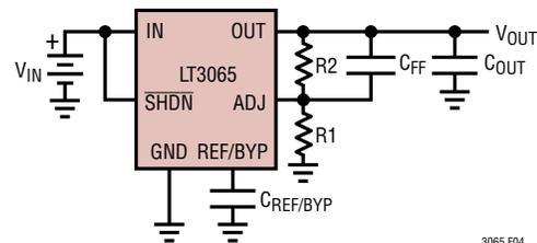
$$C_{FF} \geq \frac{10\text{nF}}{10\mu\text{A}} \cdot (I_{FB\_DIVIDER})$$
