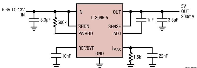
Precision Current Limit,  $R_{I_{MAX}} = 1.5k$
