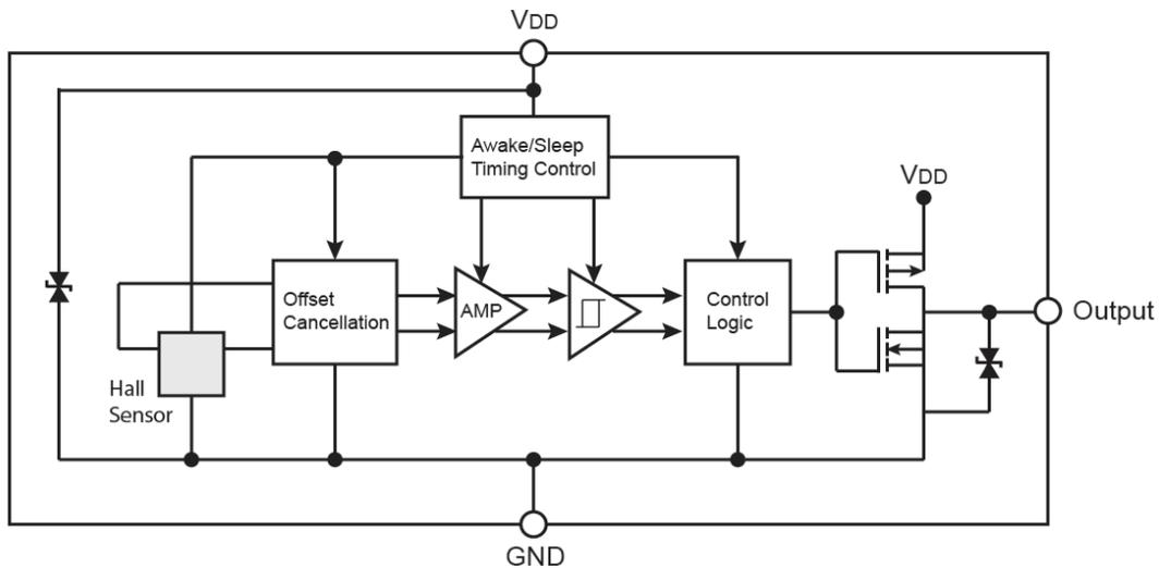
**Note:** Static sensitive device; please observe ESD precautions. Reverse VDD protection is not included. For reverse voltage protection, a 100Ω resistor in series with VDD is recommended.
