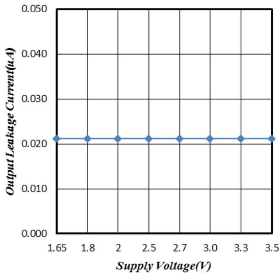
**Figure 7. Output Leakage Current vs. Supply Voltage**
