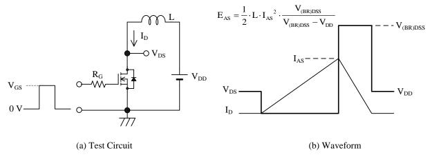
Figure 1 Unclamped Inductive Switching
