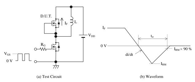
Figure 3 Diode Reverse Recovery Time
