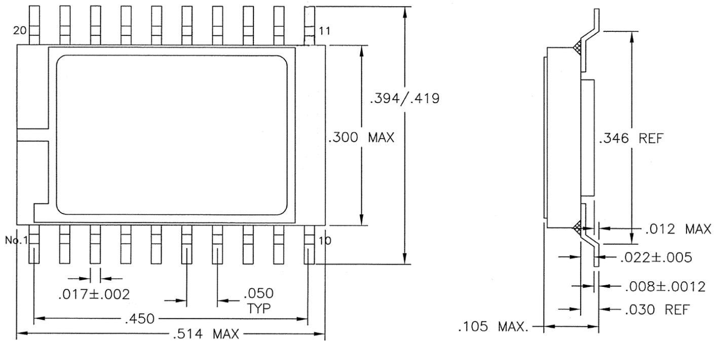
Note: Package and lid are electrically isolated from signal pads.
