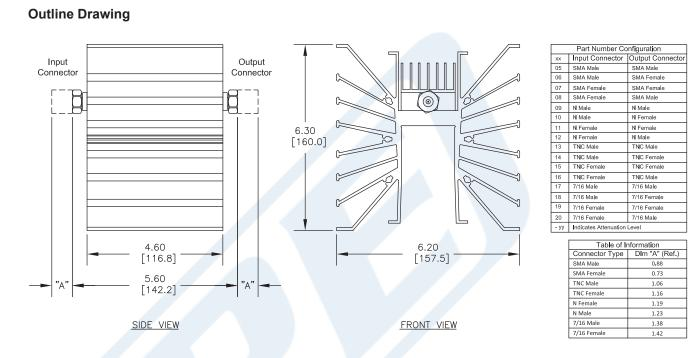
3 dB Fixed Attenuator, 7/16 DIN Male To 7/16 DIN Male Directional Black Aluminum Heatsink Body Rated To 300 Watts Up To 3 GHz from Pasternack Enterprises has same day shipment for domestic and International orders. Our RF, microwave and millimeter wave products maintain a 99% availability and are part of the broadest selection in the industry.
