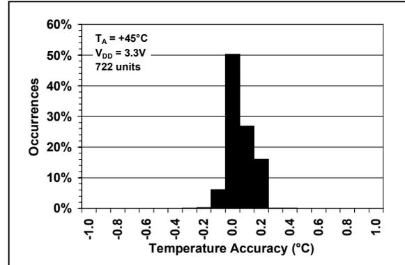
**FIGURE 2-4:** Temperature Accuracy Histogram,  $T_A = +45^{\circ}C$ .
