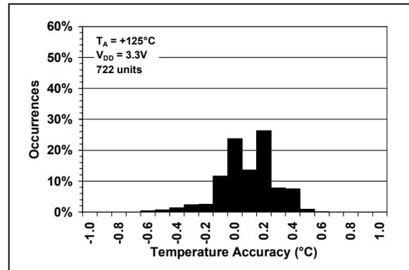
**FIGURE 2-5:** Temperature Accuracy Histogram,  $T_A = +125^{\circ}C$ .
