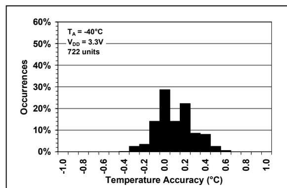
**FIGURE 2-6:** Temperature Accuracy Histogram,  $T_A = -40^{\circ}C$ .
