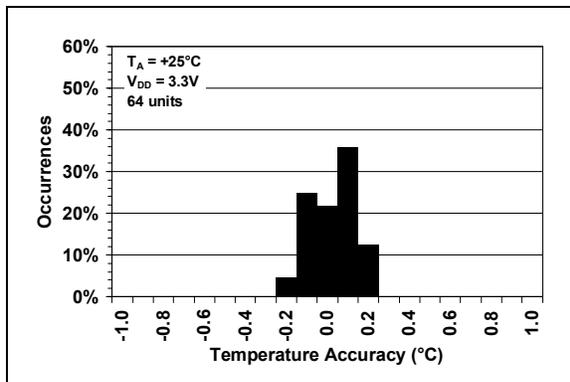
**FIGURE 2-3:** Temperature Accuracy Histogram,  $T_A = +25^{\circ}C$ .
