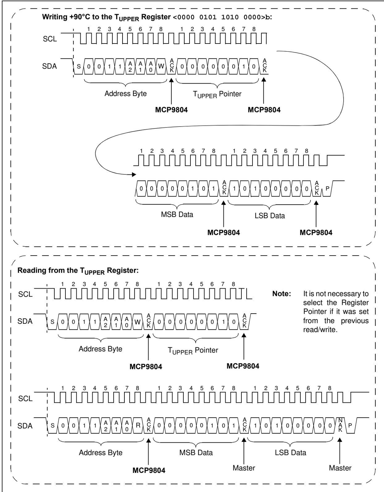
**FIGURE 5-4:** Timing Diagram for Writing and Reading from the T<sub>UPPER</sub> Register (see [Section 4.0](#) “Serial Communication”).
