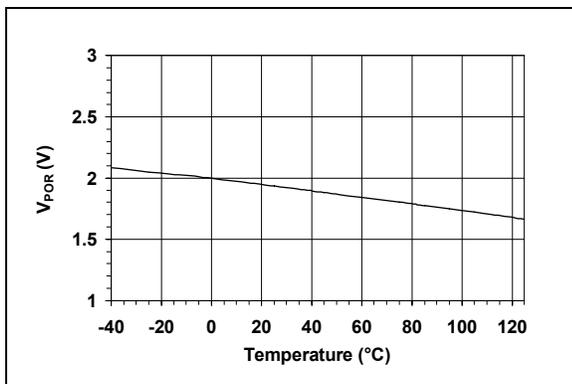
**FIGURE 2-9:** Power-on Reset Threshold Voltage vs. Temperature.
