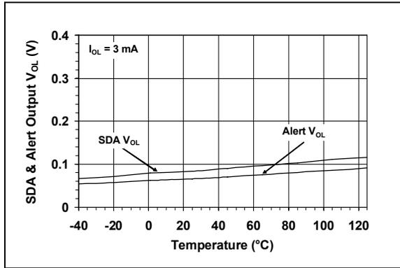
**FIGURE 2-13:** SDA and Alert Output  $V_{OL}$  vs. Temperature.
