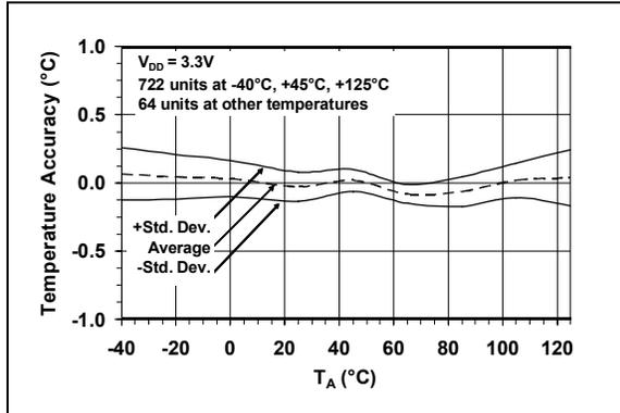
**FIGURE 2-1:** Temperature Accuracy.
