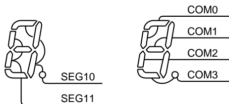
Figure 15-5 Example of COM, SEG Pin Connection (1/4 duty)
