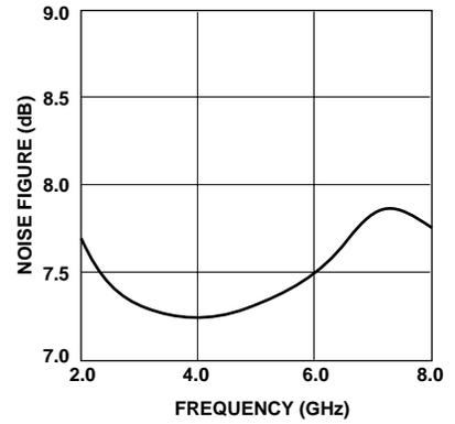
**Figure 3. Noise Figure vs. Frequency,  $V_d = 10\text{ V}$ .**
