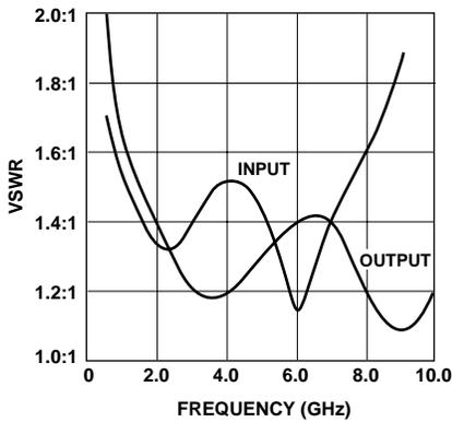
**Figure 4. VSWR vs. Frequency,  $V_d = 10\text{ V}$ .**
