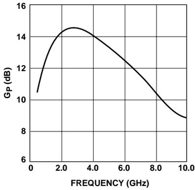
**Figure 1. Power Gain vs. Frequency,  $V_d = 10\text{ V}$ .**
