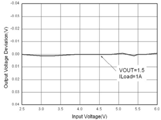
Fig. 4 Output Voltage Deviation vs Input Voltage
