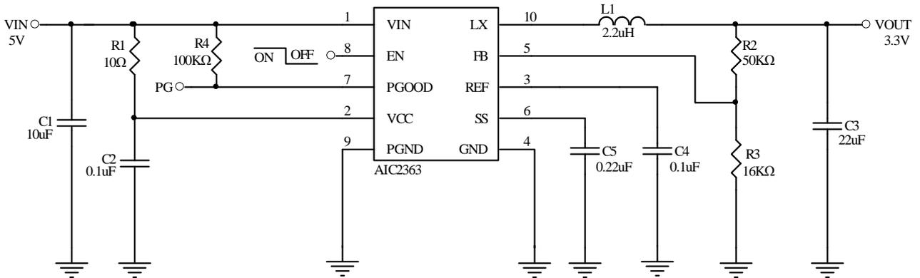
Fig. 1 Typical Application Circuit for DFN-10 Package
