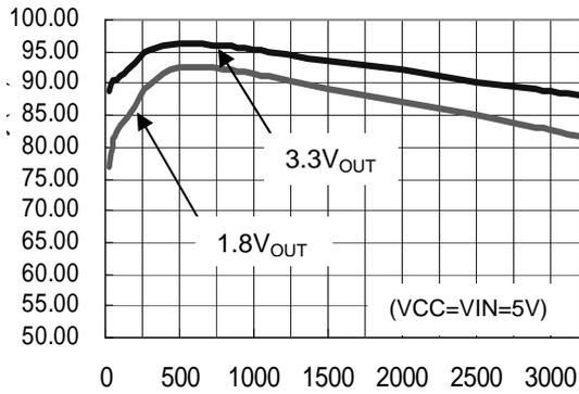
Fig. 3 Efficiency vs load Current
