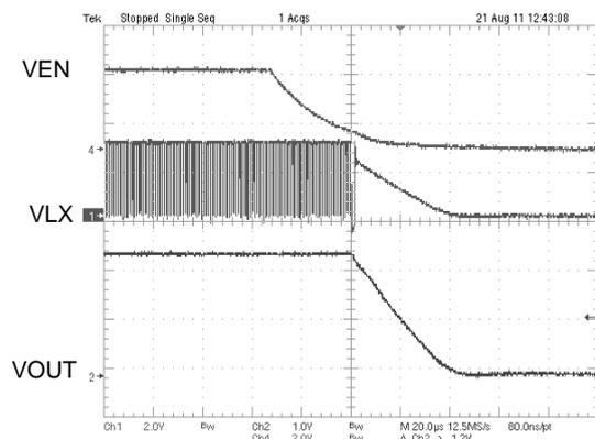
Fig. 8 Shutdown Waveform
