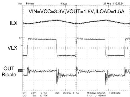
Fig. 5 Switching Waveform
