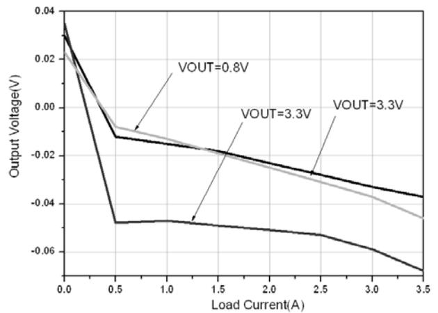
Fig. 12 Output Voltage Deviation vs Load Current
