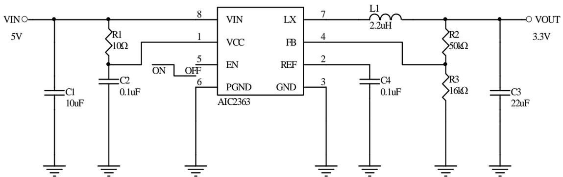
Fig. 2 Typical Application Circuit for SOP-8 Package
