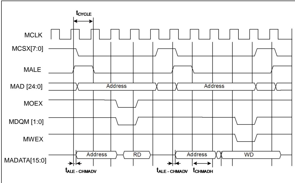
• Multiplexed Bus Access Synchronous SRAM Mode
