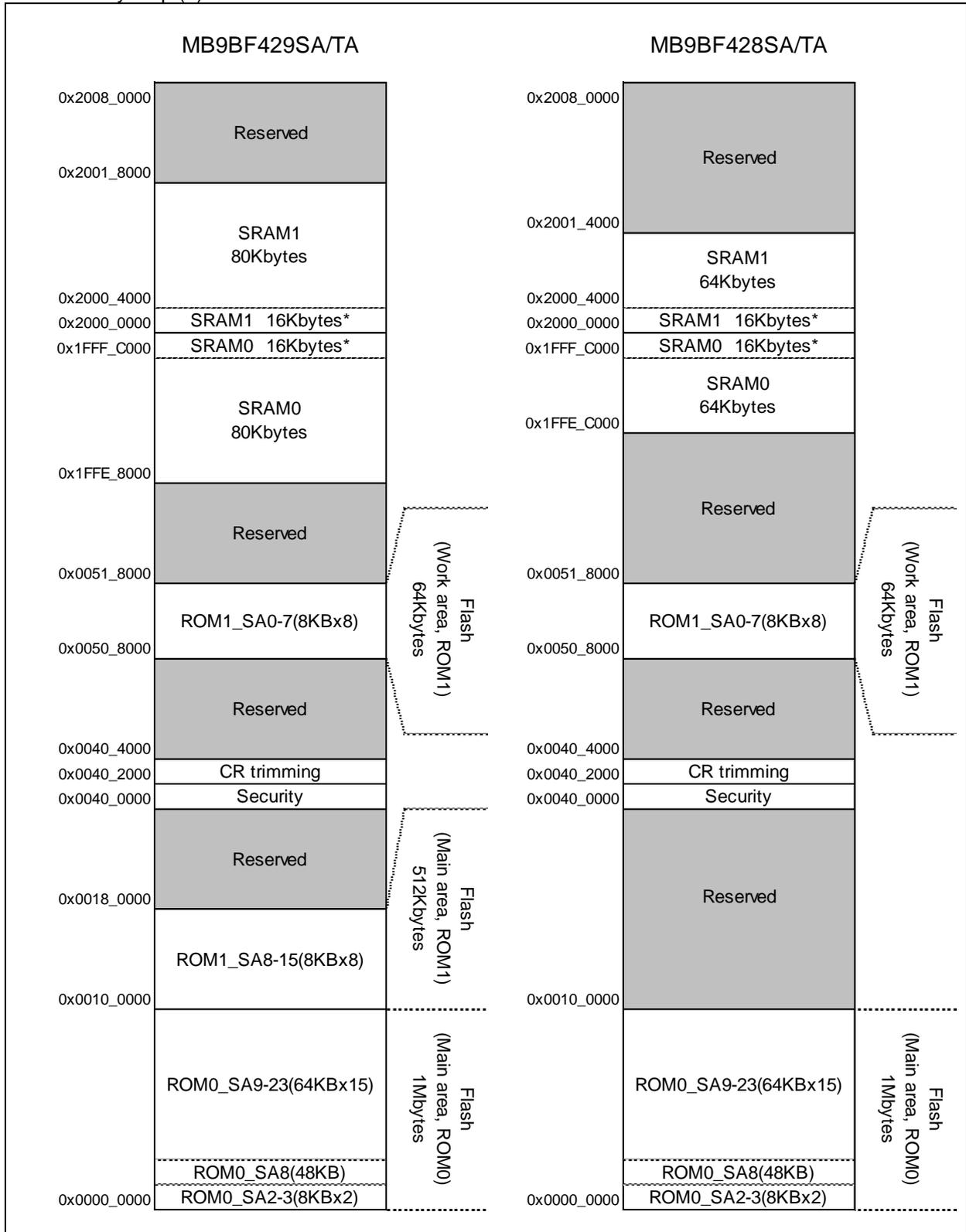
\*:The content of SRAM can be retained at the deep standby modes by the setting of Deep Standby RAM Retention Register (DSRAMR).
