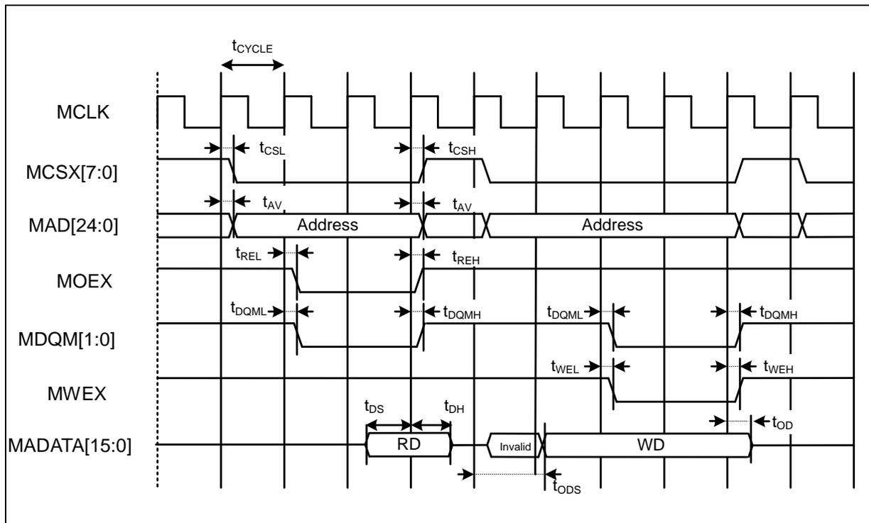
• Multiplexed Bus Access Asynchronous SRAM Mode
