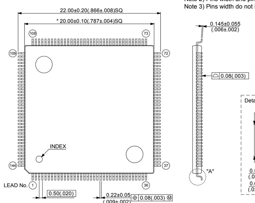
Note 1) \*:Values do not include resin protrusion.
