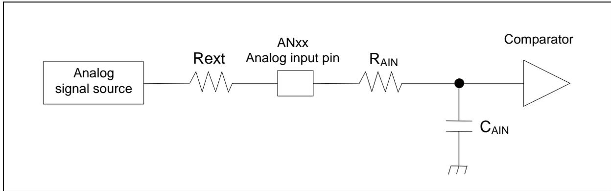
$$\text{(Equation 1) } T_s \geq (R_{AIN} + R_{ext}) \times C_{AIN} \times 9$$
