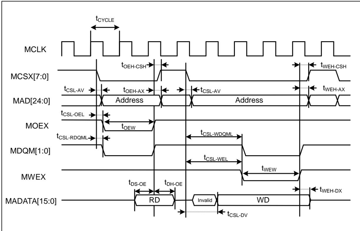
• Separate Bus Access Synchronous SRAM Mode
