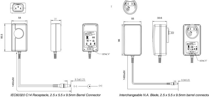
Interchangeable N.A. Blade, 2.5 x 5.5 x 9.5mm barrel connector
