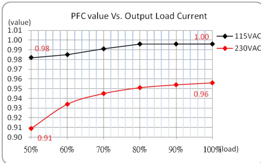
**PFC Value vs. Output Load Current (constant current mode)
