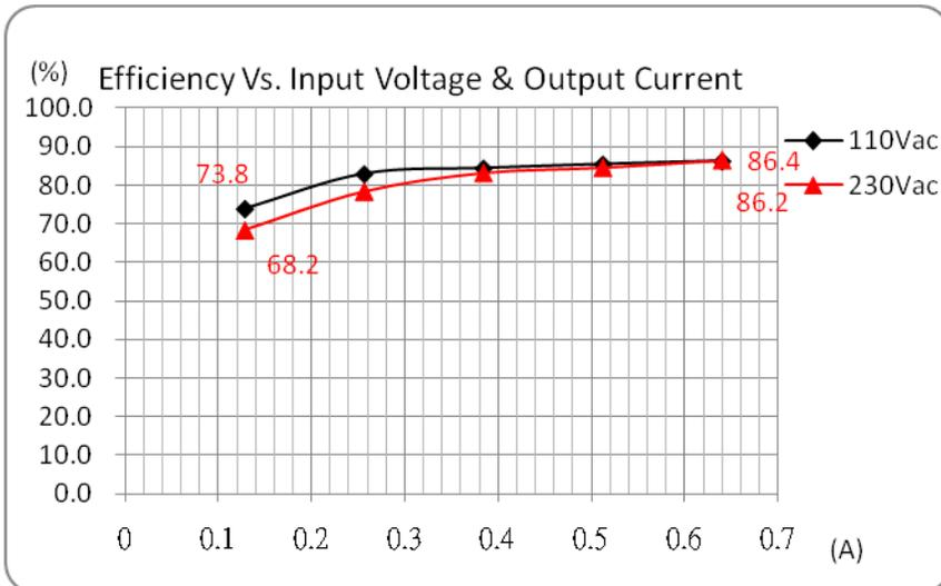
**Efficiency Vs. Input Voltage & Output Current (Constant current load)**
