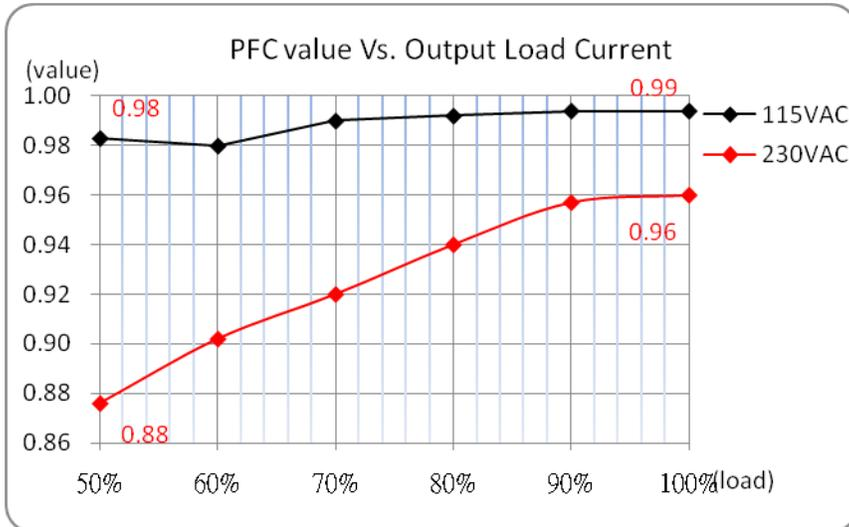
**PFC Value vs. Output Load Current (constant current mode)
