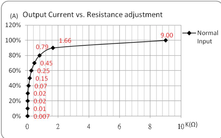
**Dimming Control (Output Current vs. Radj)
