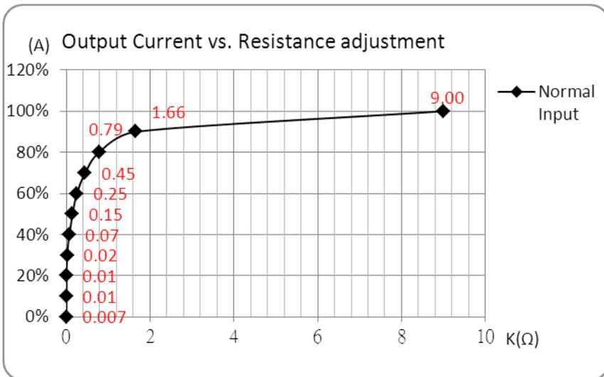
**Dimming Control (Output Current vs. Radj)
