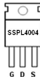
Marking and Pin Assignment
