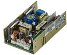
U Type (U-Chassis only): 3.2(W) x 5(L) x 1.5(H) inches.
