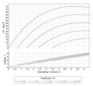
**Note**: Performance data is specified at optimal conditions (TEC hot side is stabilized at ambient temperature). Heatsink thermal resistance is not included into estimations. Use TECCad Software for estimations under different conditions.
