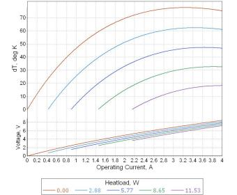
**Note**: Performance data is specified at optimal conditions (TEC hot side is stabilized at ambient temperature). Heatsink thermal resistance is not included into estimations. Use TECCad Software for estimations under different conditions.
