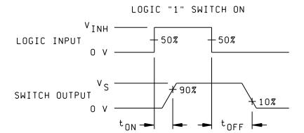
NOTE: For device types 01, 03, 04, 05, 06, 07, and 08,  $V_{INH}$  = +4 V. For device type 02,  $V_{INH}$  = +15 V. For device types 01, 02, 03, 04, 06, and 08, V- = -15 V and V+ = +15 V. For device types 05 and 07, V- = -12 V  $\pm$ 10 % and V+ = +12 V  $\pm$ 10 %.
