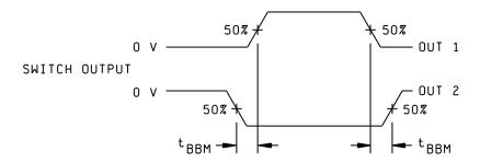
NOTE: For device types 01, 03, 04, 05, 06, 07, and 08,  $V_{INH}$  = +5 V. For device type 02,  $V_{INH}$  = +15 V. For device types 01, 02, 03, 04, 06, and 08, V- = -15 V and V+ = +15 V. For device types 05 and 07, V- = -12 V  $\pm$ 10 % and V+ = +12 V  $\pm$ 10 %.
