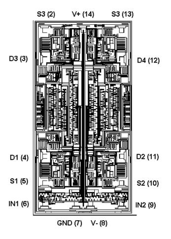
NOTE: Pad numbers reflect terminal numbers when placed in case outlines C and X (see figure 1).
