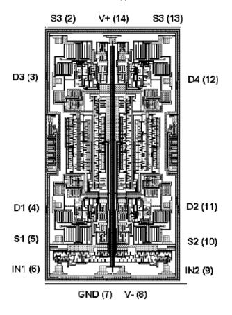
NOTE: Pad numbers reflect terminal numbers when placed in case outlines C and X (see figure 1).
