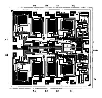
NOTE: Pad numbers reflect terminal numbers when placed in case outlines E and Y (see figure 1).
