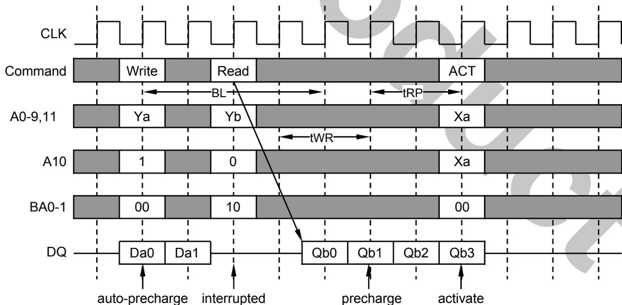
**Read with Auto-Precharge Interrupted by Read to Different Bank**
