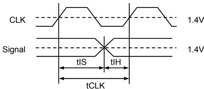
AC timing is referenced to the input signal crossing through 1.4V.
