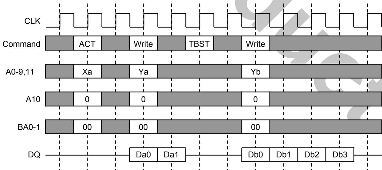
**Write with Auto-Precharge Interrupted by Write / Read to Different Bank**
