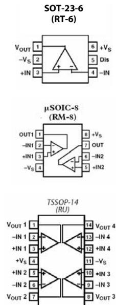
The ADA4851 also has high output current making them ideal in driving video signals. The ADA4851-1 contains a disable feature that will lower the power of the amplifier and put the output in high impedance mode which makes it possible for muxing applications.
