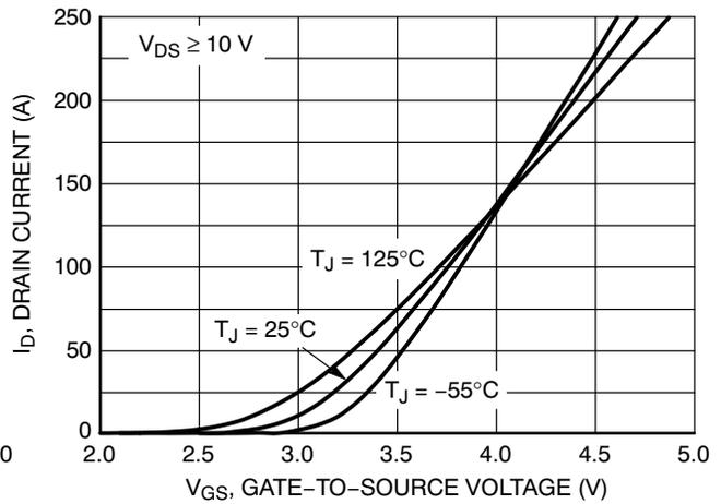
Figure 2. Transfer Characteristics
