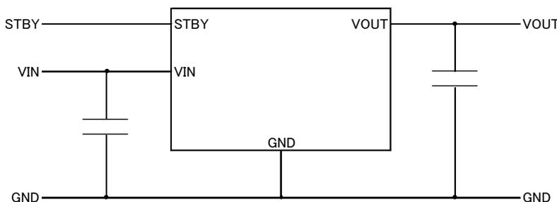
Figure 1. Application Circuit
