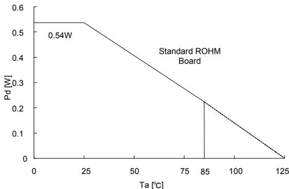
\* Please design the margin so that P<sub>MAX</sub> becomes is than Pd (P<sub>MAX</sub><Pd) within the usage temperature range
