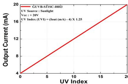
$$\text{UV Index (UVI)} = [I_{\text{out}} (\text{mA}) - 4] \times 1.25$$
