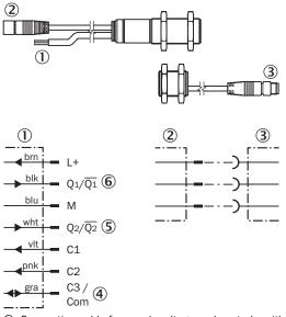
① Connection cable for supply voltage and controls, with control inputs C1, C2, C3 and switching output Q1, Q2
