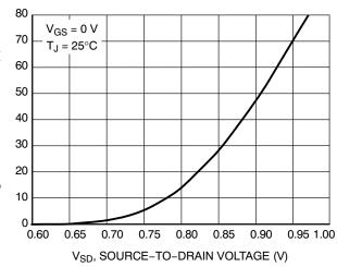
Figure 10. Diode Forward Voltage vs. Current
