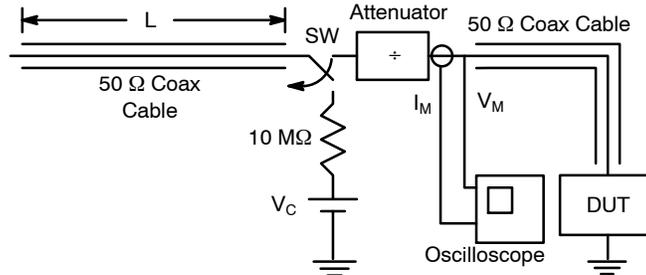
Figure 5. Simplified Schematic of a Typical TLP System
