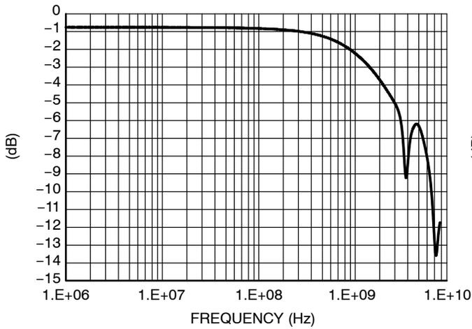
Figure 1. Differential Mode Attenuation vs. Frequency
