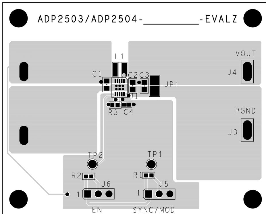
Figure 31. ADP2503/ADP2504 Evaluation Board for Fixed Output Voltages
