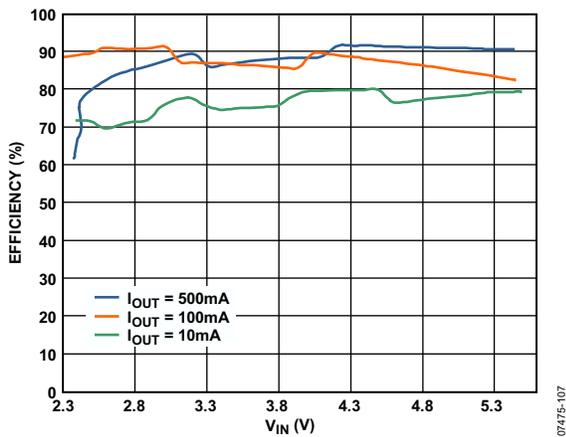
Figure 11. Efficiency vs. Input Voltage ( $V_{OUT} = 3.3\text{ V}$ )
