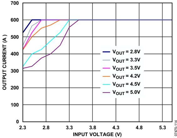
Figure 3. ADP2503 Output Current vs. Input Voltage
