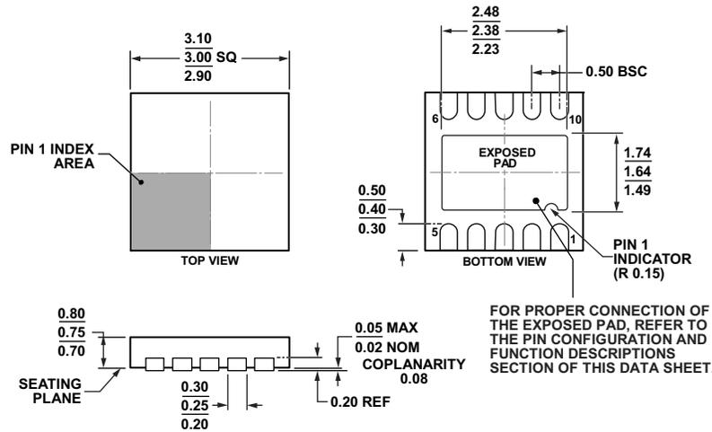
Figure 32. 10-Lead Lead Frame Chip Scale Package [LFCSP\_WD]
