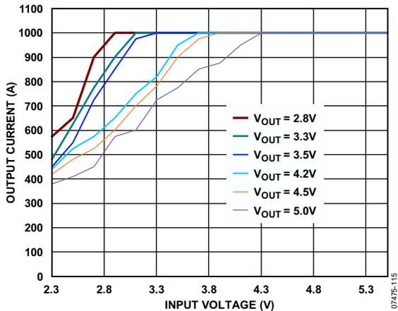
Figure 4. ADP2504 Output Current vs. Input Voltage
