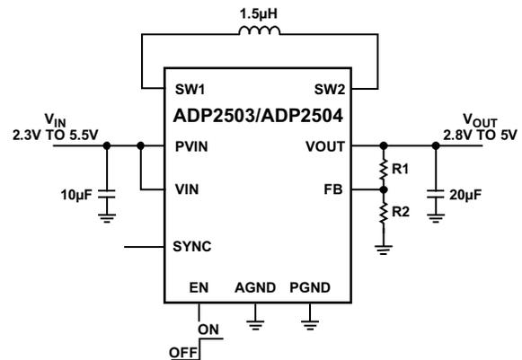
Figure 30. Typical Application Circuit for the Adjustable ADP2503/ADP2504
