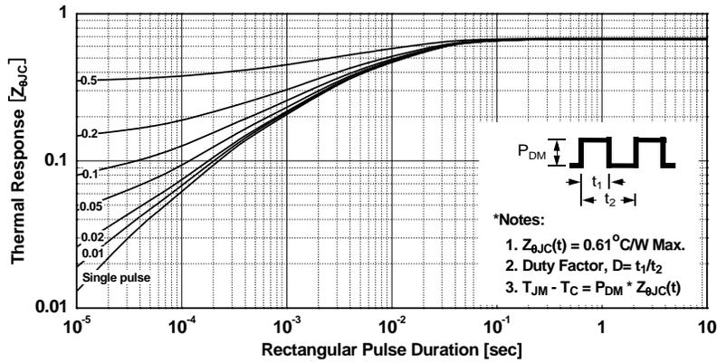
Figure 13. Transient Thermal Response Curve - FCPF22N60NT
