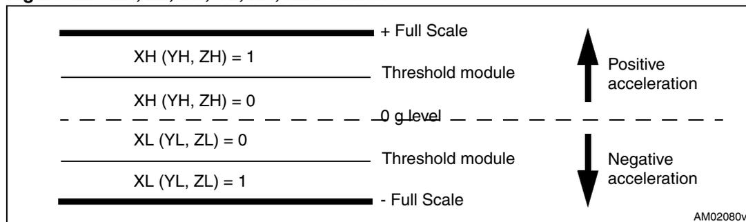
There are two possible configurations for the 6D direction function:
