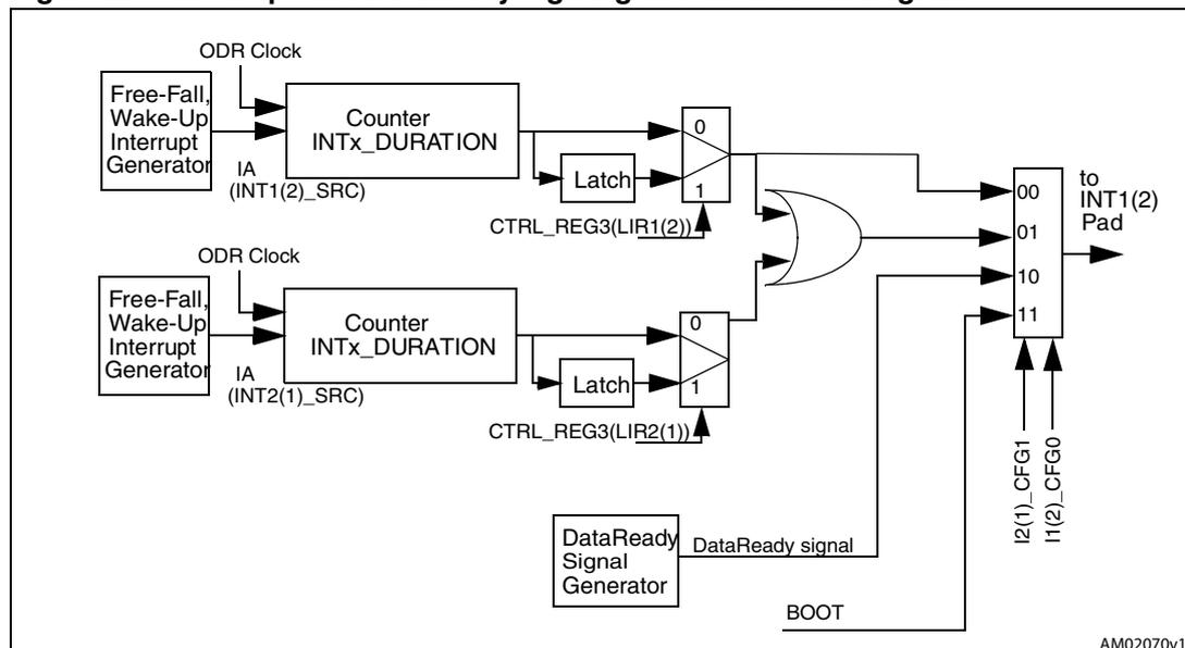
In particular, the data-ready (DR) signal rises to 1 when a new set of acceleration data has been generated and is available for reading. The signal is reset after all the enabled channels are read through the serial interface.
