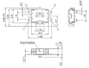
Parts indicated by \* apply only to products with a ground terminal.
