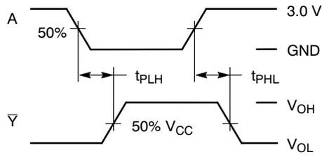
**Figure 4. Switching Waveforms**
