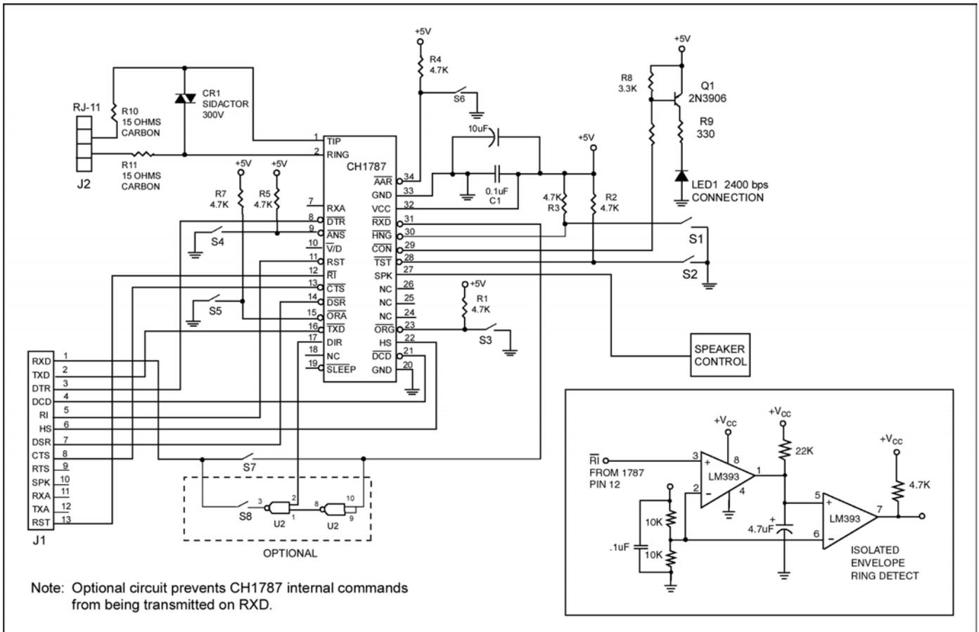
Figure 4. CH1787 Application Diagram of Test Circuit.
