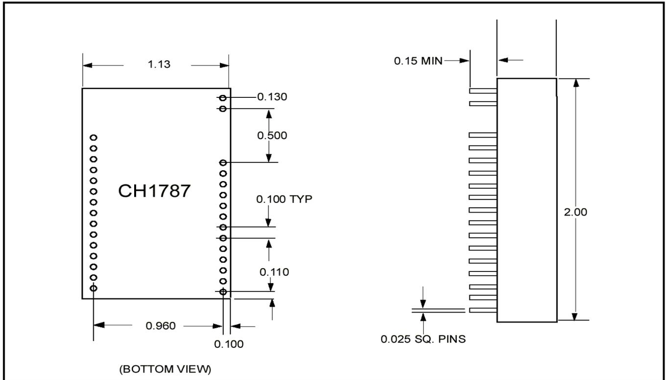
Figure 7. CH1787 Physical Dimensions and Pin Functions.
