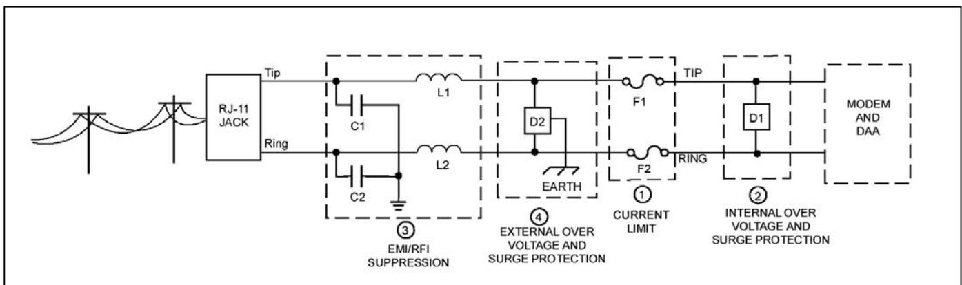
Figure 6. Telephone Interfaces.
