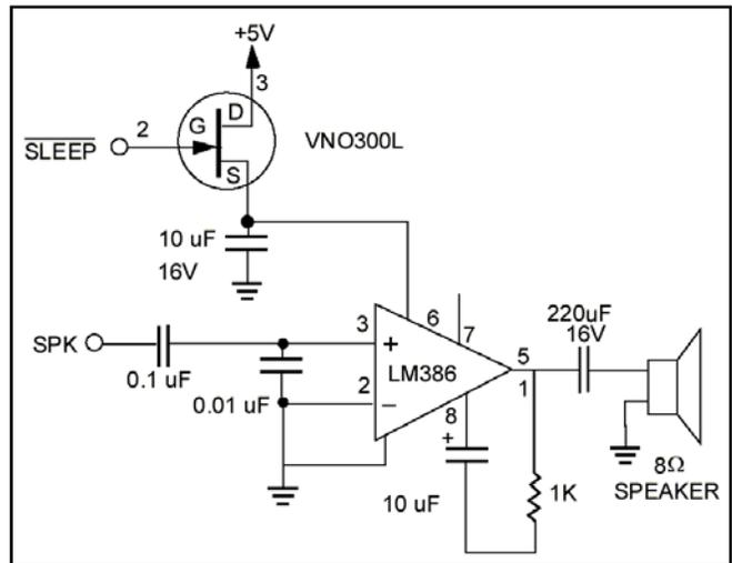
**Figure 5. Speaker Control. Circuit allows call progress monitoring.**
