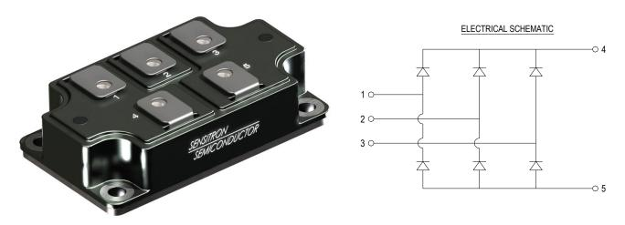
DESCRIPTION: 1200 V, 200 A THREE PHASE BRIDGE RECTIFIER ASSEMBLY MAX. RATINGS / ELECTRICAL CHARACTERISTICS All ratings are at  $T_A = 25^{\circ}$ C unless otherwise specified.
