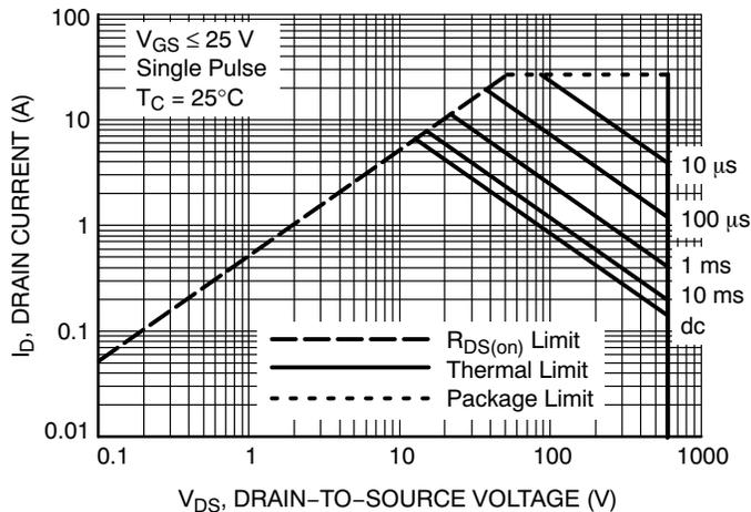
Figure 13. Maximum Rated Forward Biased Safe Operating Area
