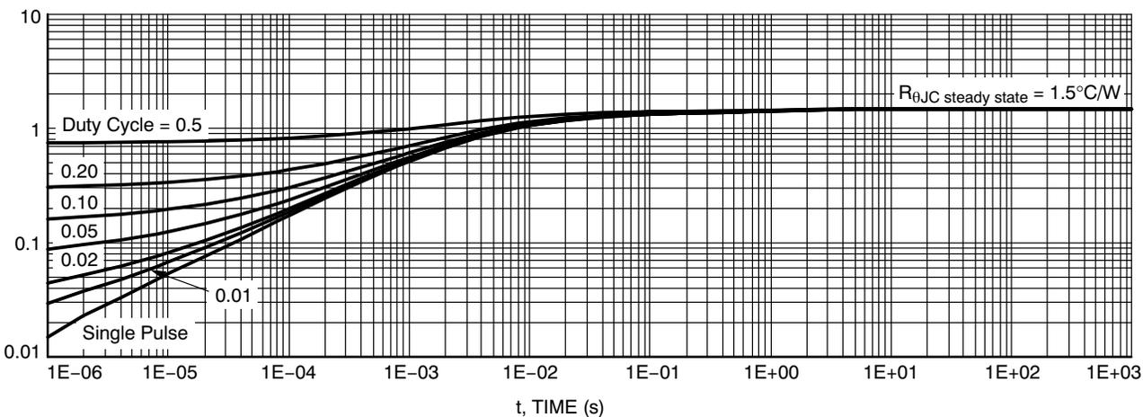
Figure 14. Thermal Impedance (Junction-to-Case)
