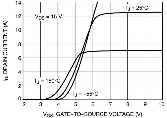
Figure 2. Transfer Characteristics
