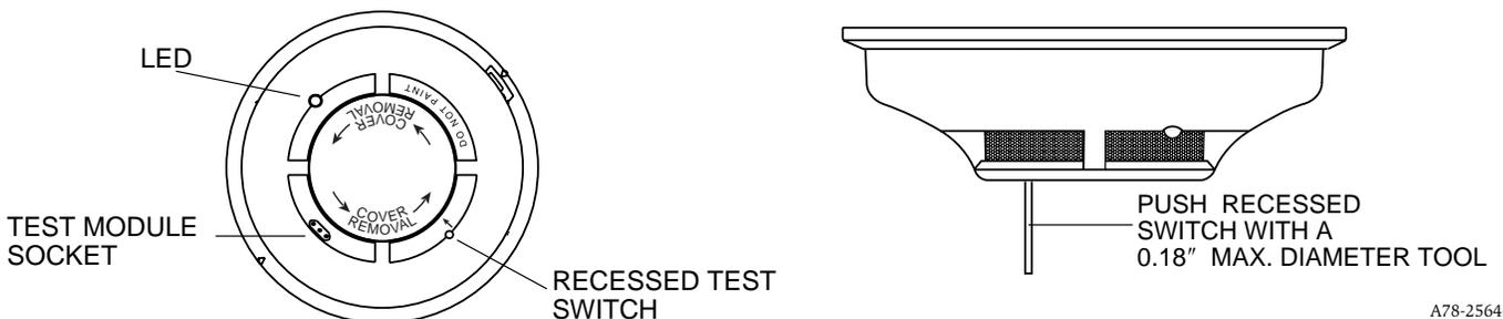
1. Remove cover by turning counter clockwise in direction of arrow.
