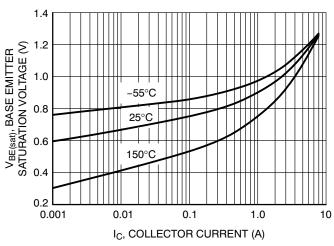
Figure 4. Base Emitter Saturation Voltage vs.
