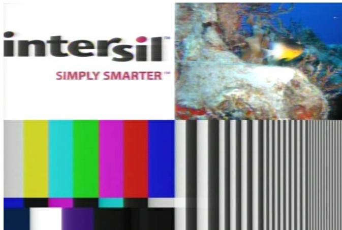
FIGURE 29. TEST PATTERN IMAGE AFTER 3000 FEET OF UNCOMPENSATED RG-59 COAX
