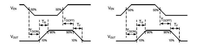
Figure 1 Voltage Waveforms: AP2141D (left), AP2151D (right)
