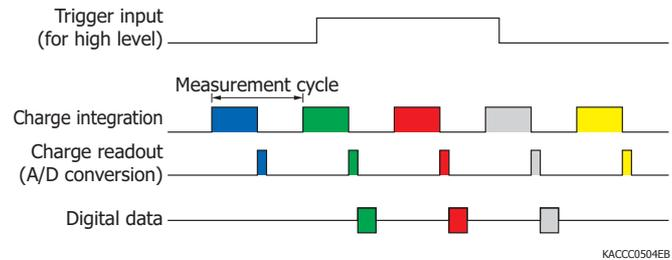
(6) Synchronous data measurement at external trigger input level
