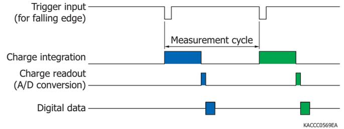
(5) Asynchronous data measurement at external trigger input level
