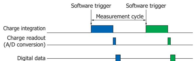
(3) Asynchronous data measurement at external trigger input
