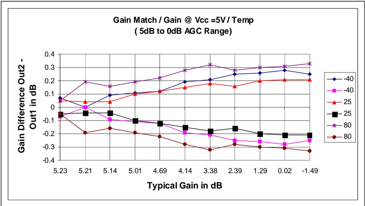
Figure 18 - Typical Gain Matching / AGC @ 5V Vcc / Temp
