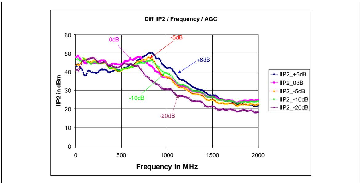
Figure 24 - Typical Differential IIP2 / Frequency / AGC Setting
