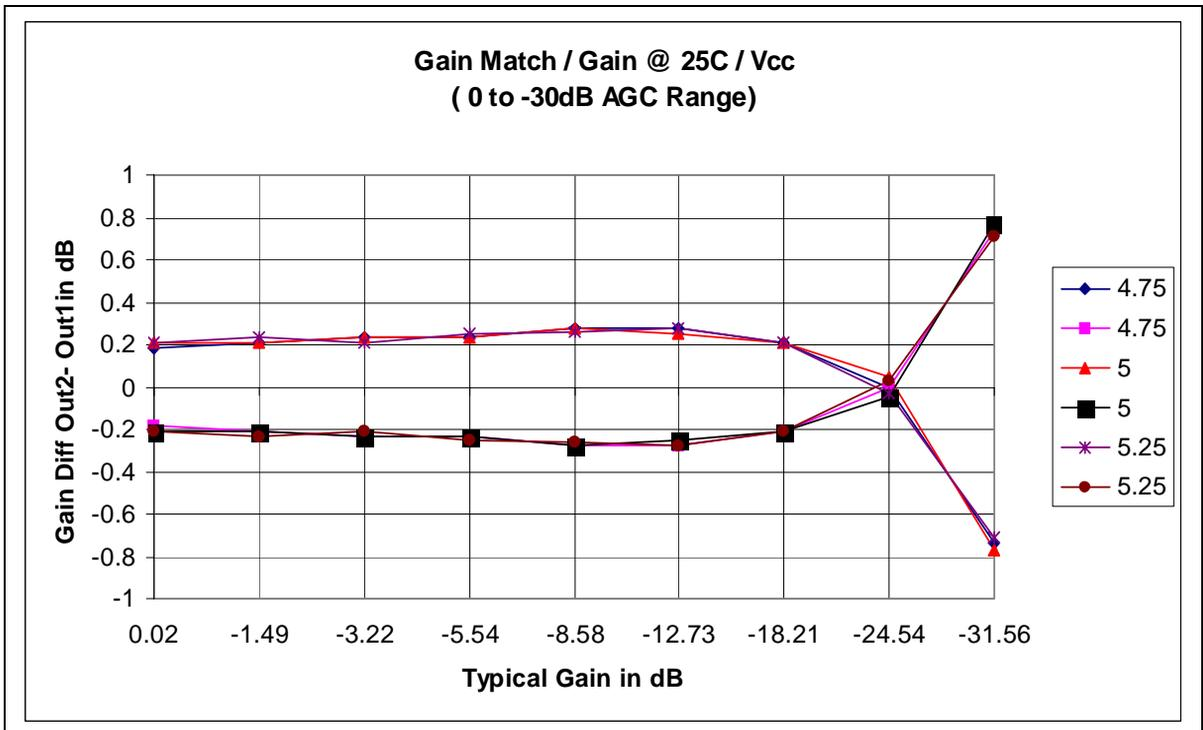
Figure 17 - Typical Gain Match 1 to 2 / Gain @ 25C / Vcc
