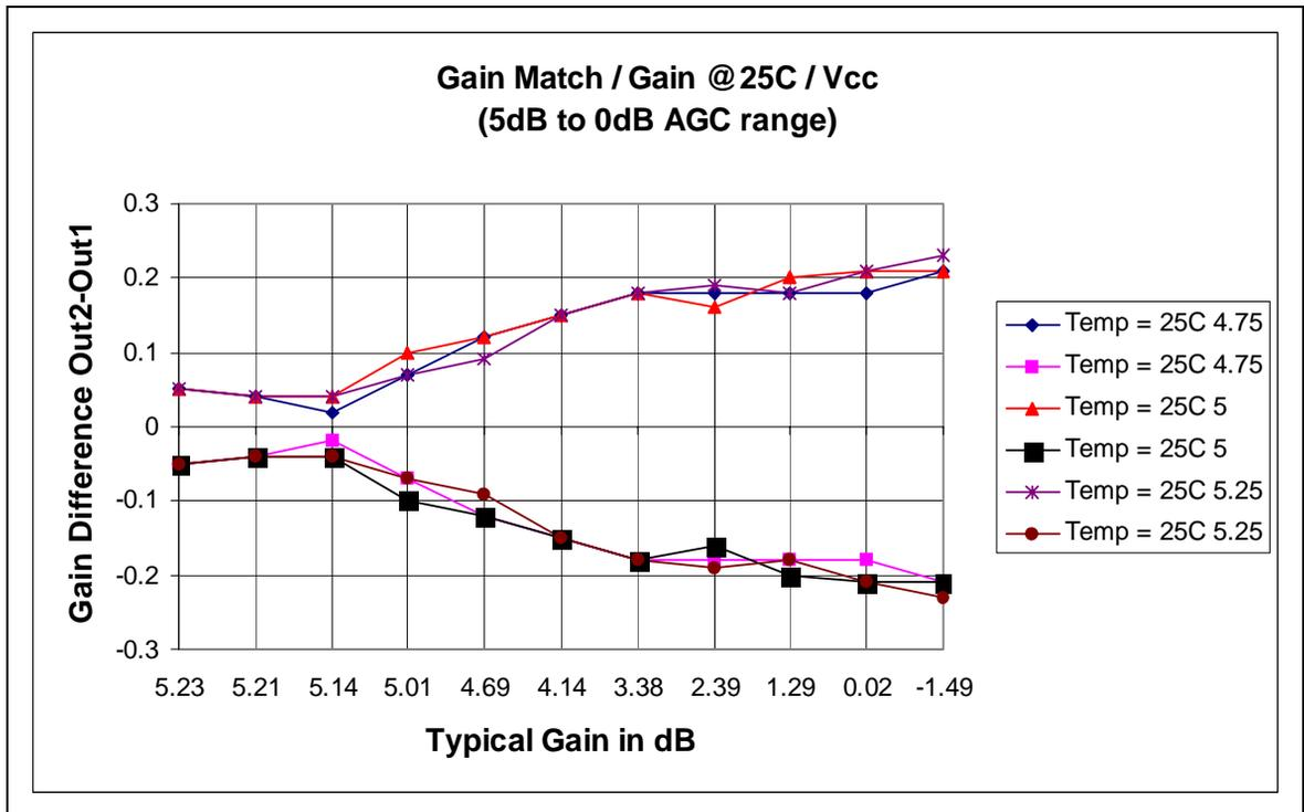
Figure 16 - Typical Gain Matching / AGC @ 25C / Vcc
