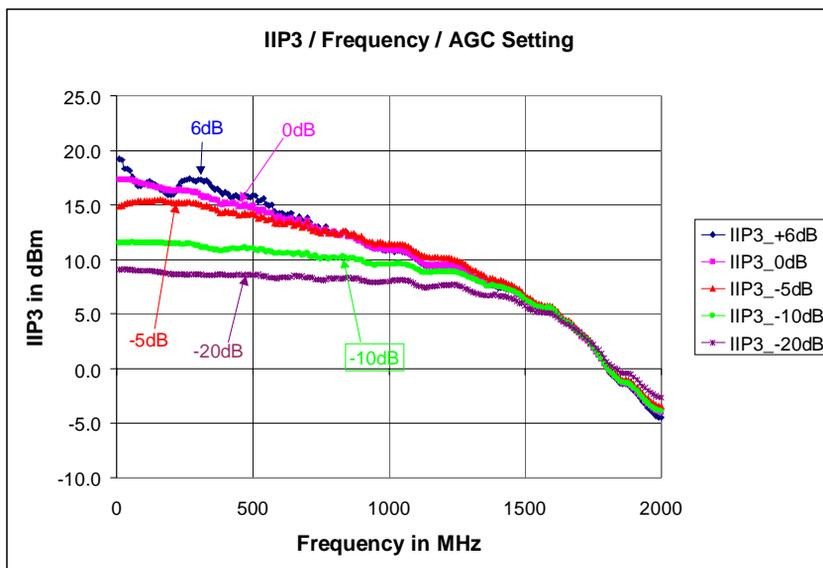
Figure 30 - Typical IIP3 @ Max Gain Differential / Frequency
