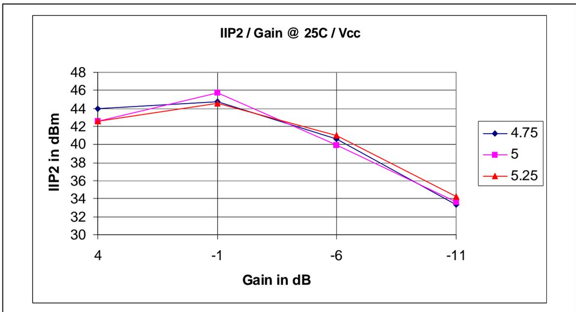
Figure 22 - Typical IIP2 / Gain @ 25C / Vcc @ 500MHz
