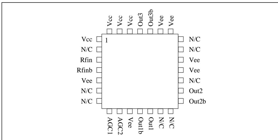
Figure 2 - Pin Diagram
