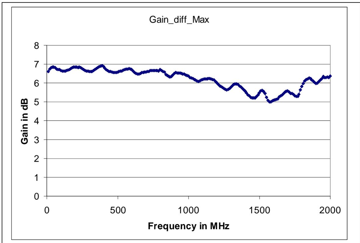
Figure 10 - Typical Diff Max Gain / Frequency
