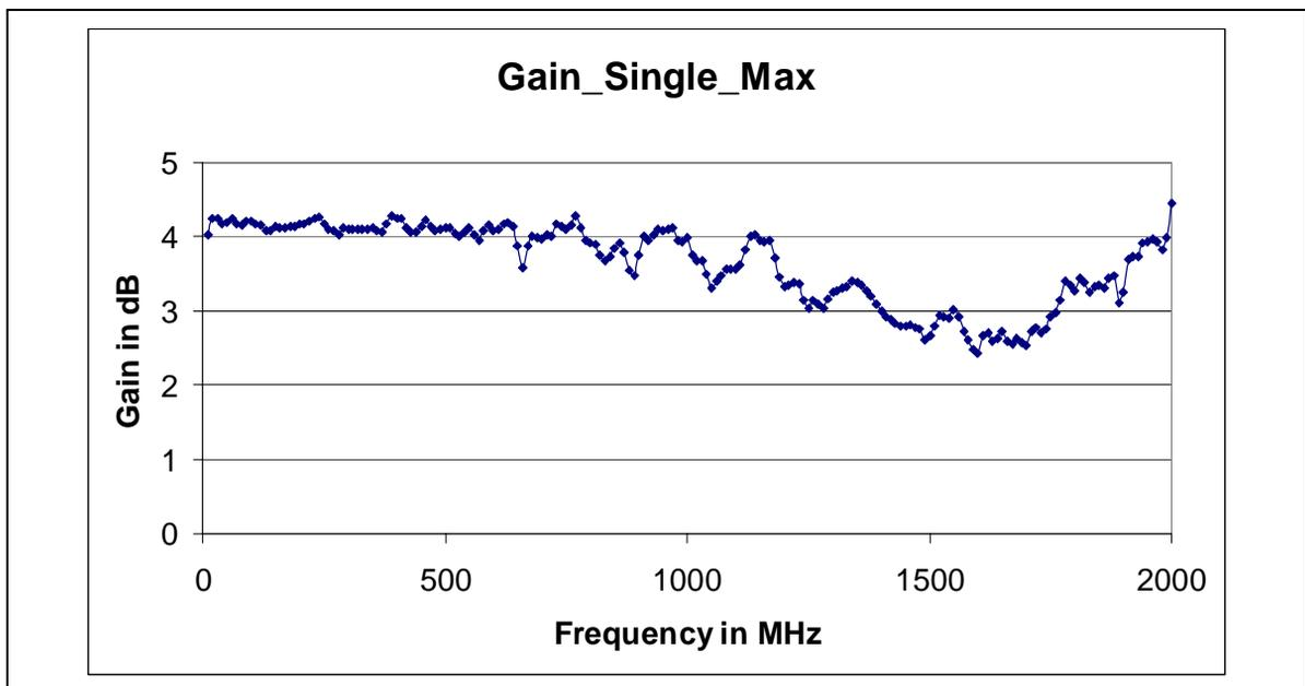
Figure 11 - Typical Single Ended Max Gain / Frequency
