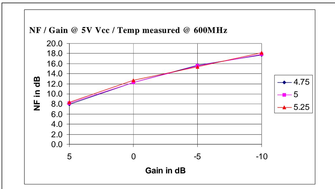
Figure 34 - Typical Differential NF / Gain @ 5V Vcc / Temp measured @ 600MHz
