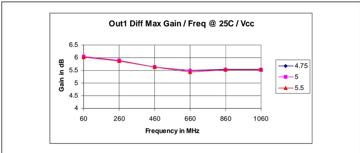
Figure 6 - Typical Ch1&2 Diff Gain / Freq / Vcc @ 25C
