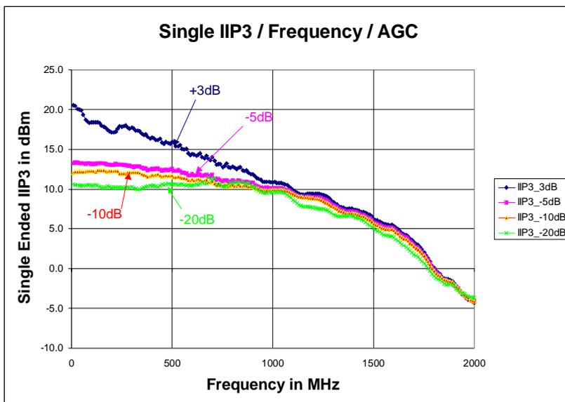
Figure 31 - Typical IIP3 Single Ended / Frequency / AGC
