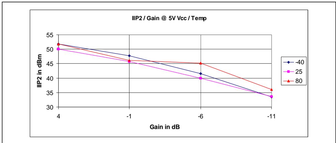
Figure 23 - Typical IIP2 / Gain @ 5V Vcc / Temp @ 500MHz
