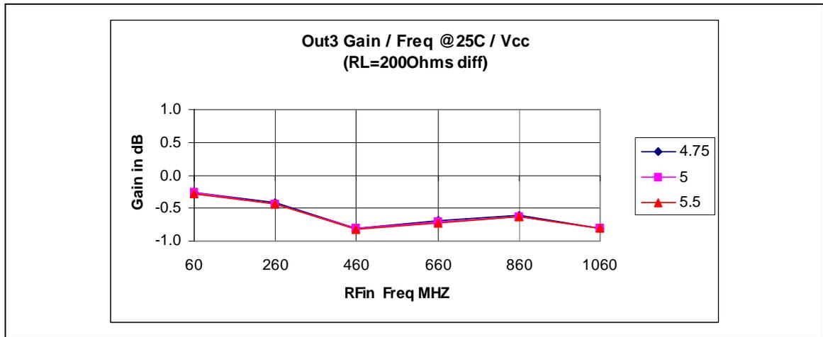
Figure 7 - Typical Ch3 Diff Gain / Freq / Vcc @ 25C
