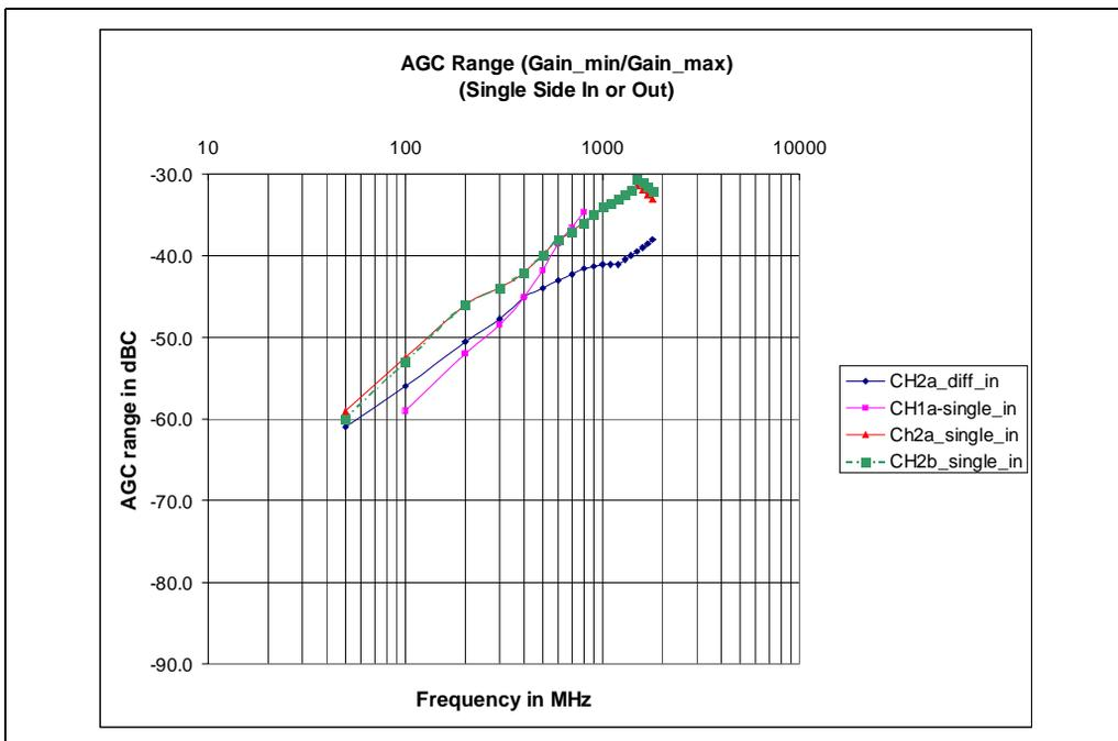
Figure 15 - Typical AGC Range / Frequency (Single Ended output)
