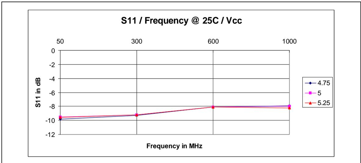
Figure 36 - Typical S11 in 50Ohm System
