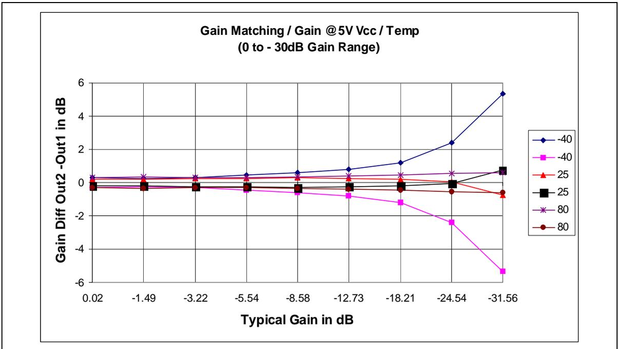
Figure 19 - Typical Gain Matching / AGC @ 5V Vcc / Temp
