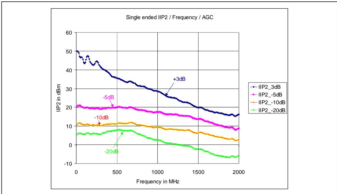
Figure 25 - Typical Single Ended IIP2 / Frequency / AGC
