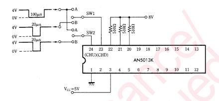
$\bigcirc$ SW1 and SW2 at the side A are initialized in a pulse of 100  $\mu$ s.
