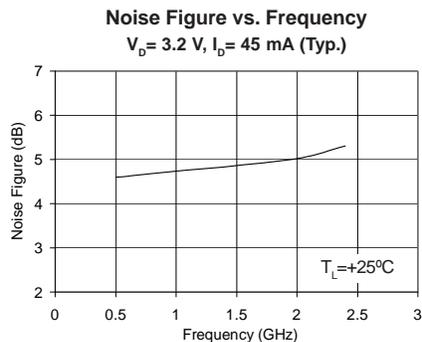
**Typical RF Performance Over Temperature ( Bias:  $V_D = 3.2$  V,  $I_D = 45$  mA (Typ.) )**
