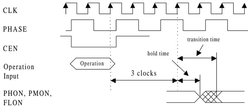
Fig. 9.4.4 Output cycle of PHON, PMON, and FLON
