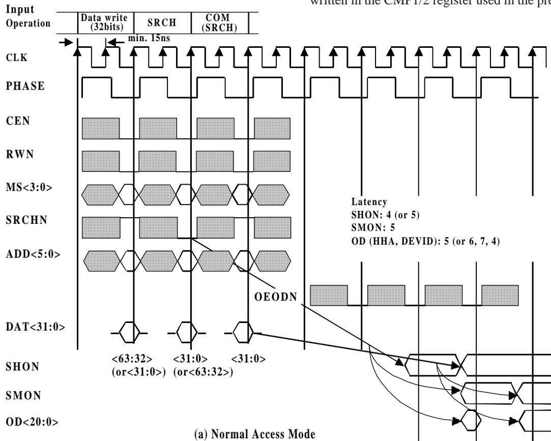
Fig. 4.4.1 SRCH Operation through CMP Register Write
