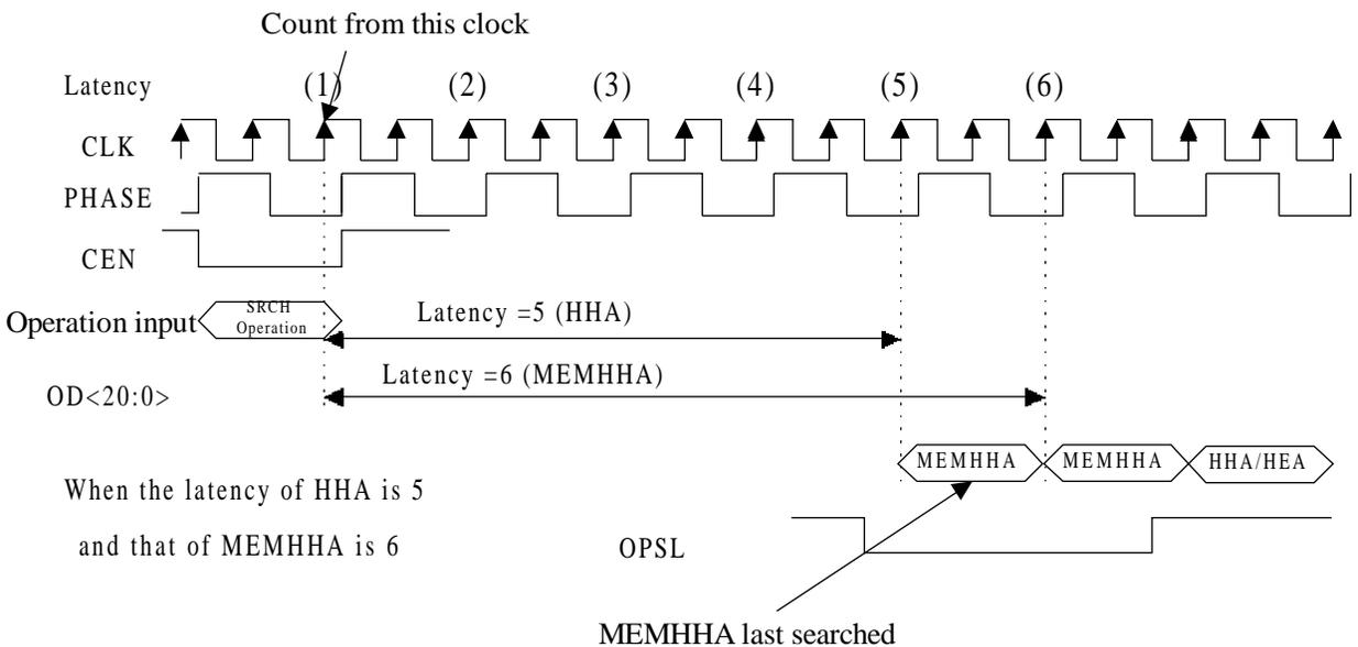
Fig. 5.3.4.1(b) Timing of the Output Condition
