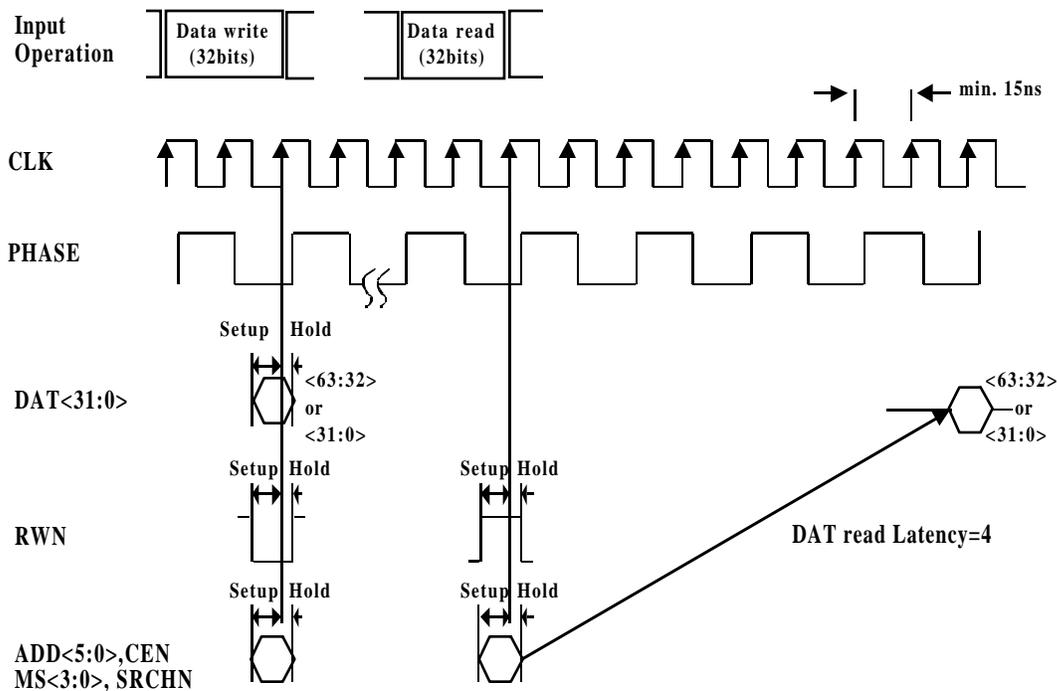
Fig. 4.1.1 (a) CPU Access Mode (Normal Access Mode)
