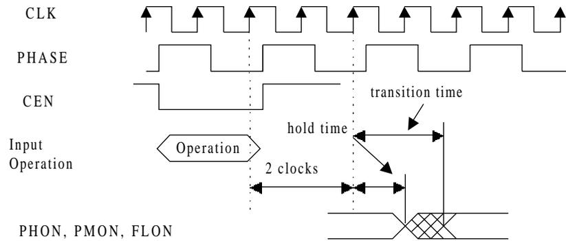
Fig. 9.4.5 Output cycle of PHON, PMON, and FLON
