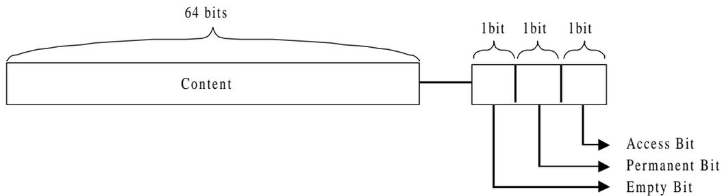
Fig.4.3.1 Word Structure of CAM
