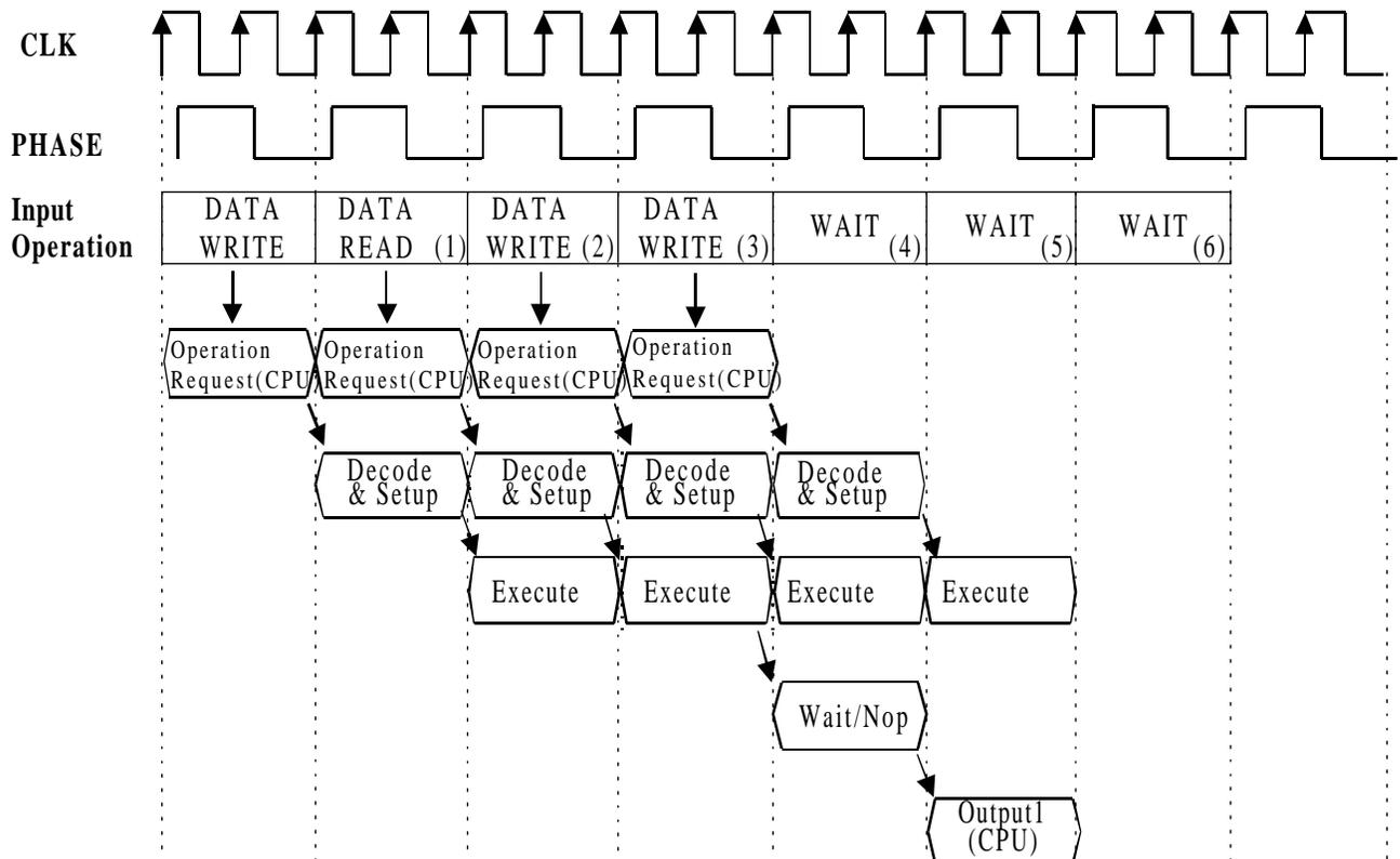
Fig.4.6.2 Restrictions between Data Read/Write Operations
