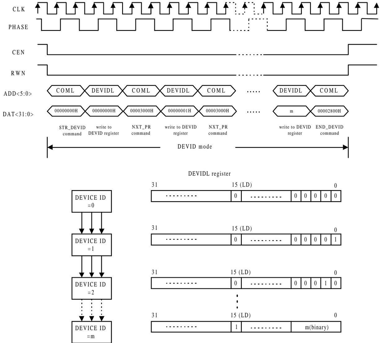
Fig.5.3.1.2 Device ID registration procedure
