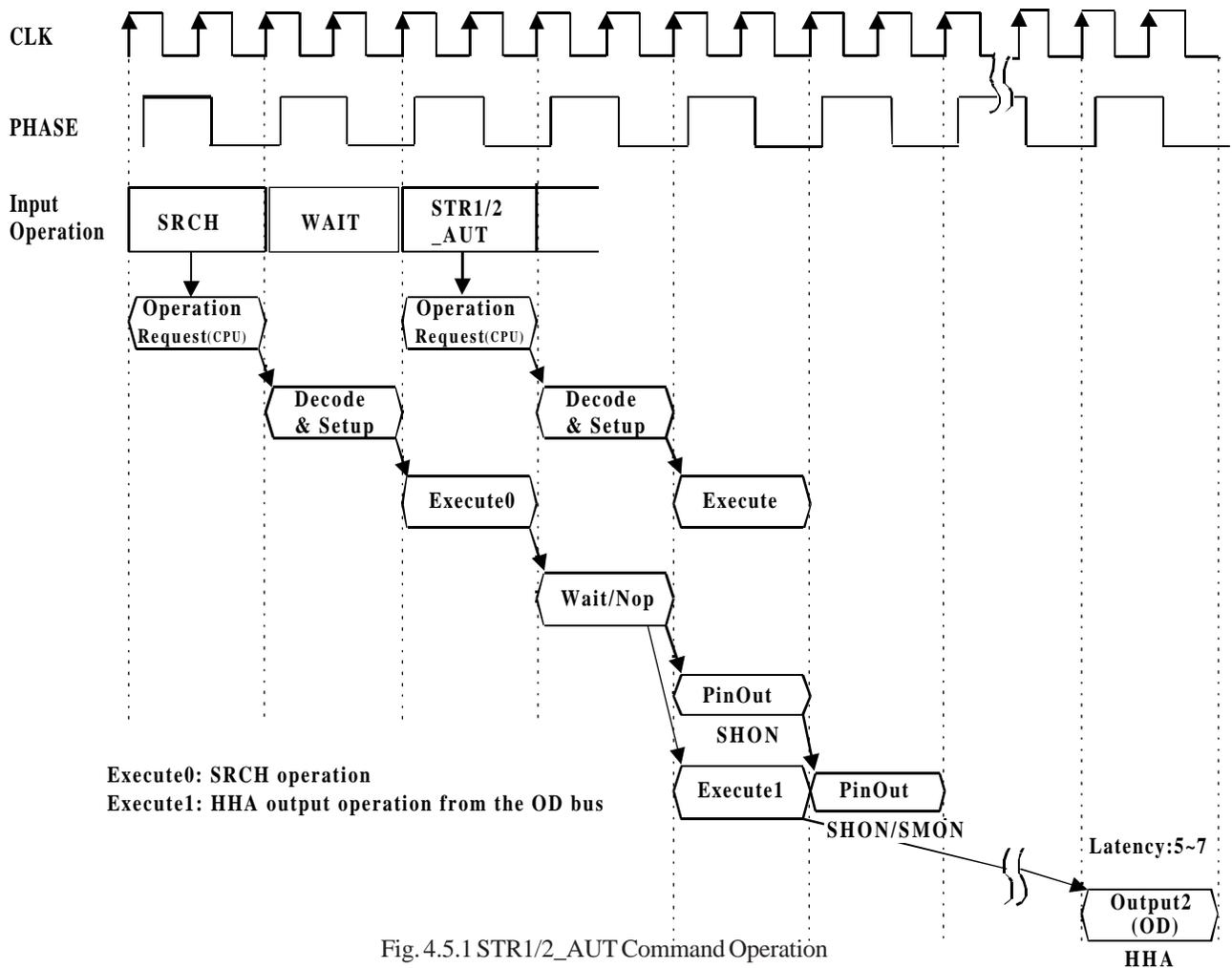
Fig. 4.5.1 STR1/2\_AUT Command Operation
