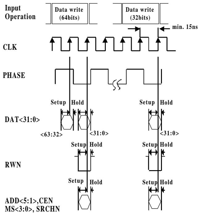
Fig. 4.1.1 (b) CPU Access Mode (Fast Write Mode)
