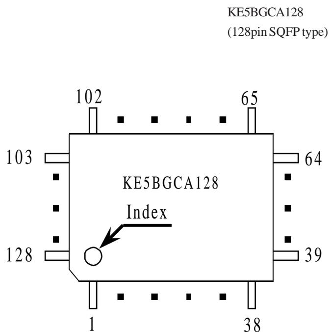
Fig. 3.1.1 Pin Assignment
