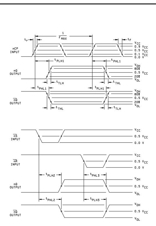
FIGURE 4. Switching waveforms and test circuit.
