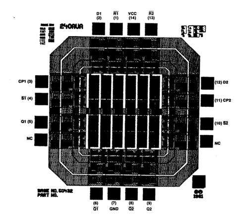
Note: Pad numbers reflect terminal numbers when placed in case outlines C and X (see figure 1).
