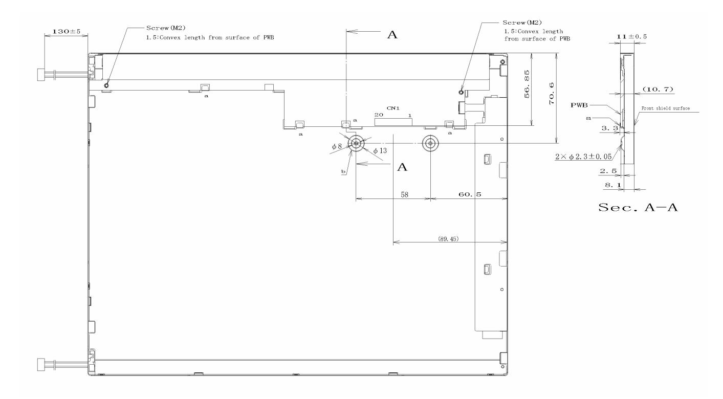
Note1: The values in parentheses are for reference. Note2: Not shown tolerances of the dimensions are  $\pm 0.5$  mm. Note3: The torque for mounting screws must never exceed 0.343N·m.
