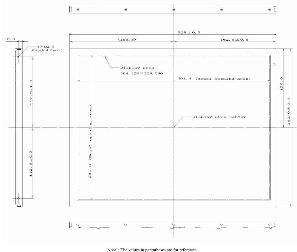
Note2: Not shown tolerances of the dimensions are  $\pm 0.5$  mm. Note3: The torque for mounting screws must never exceed 0.343N·m.
