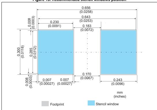
Figure 13. Recommended stencil windows position
